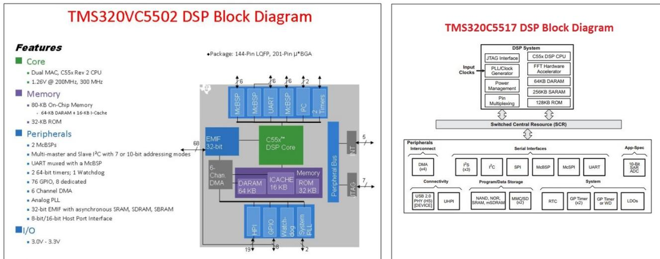
Figure 1. TMS320VC5502 and TMS320C5517 DSP Block Diagrams
