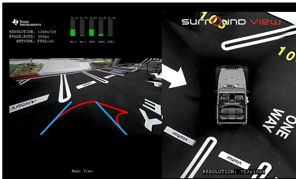
Figure 1-5. Display Output of Algorithm Running on TDA3x
