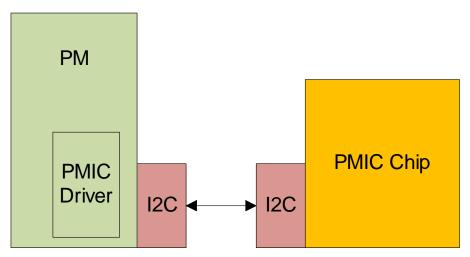
Figure 2. SOC-PMIC Communication Over I2C Bus
