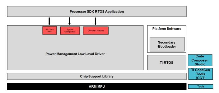
Figure 1. Power Management Software Stack
