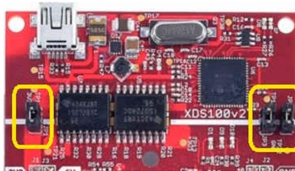
**Figure 2-6. F28379D Jumper Configuration**
