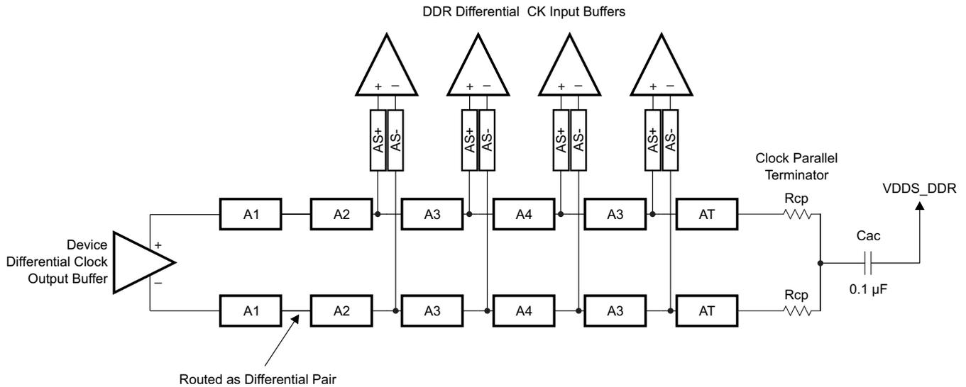
Figure 3. CK Topology for Four DDR3 Devices
