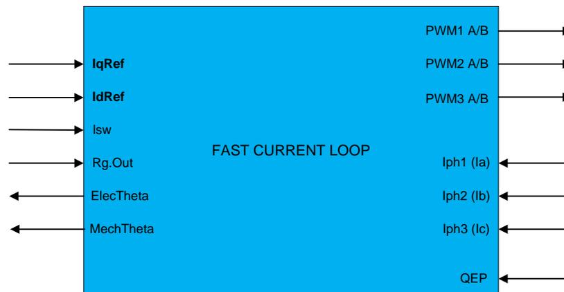
**Figure 2. Fast Current Loop Library Block Diagram**
