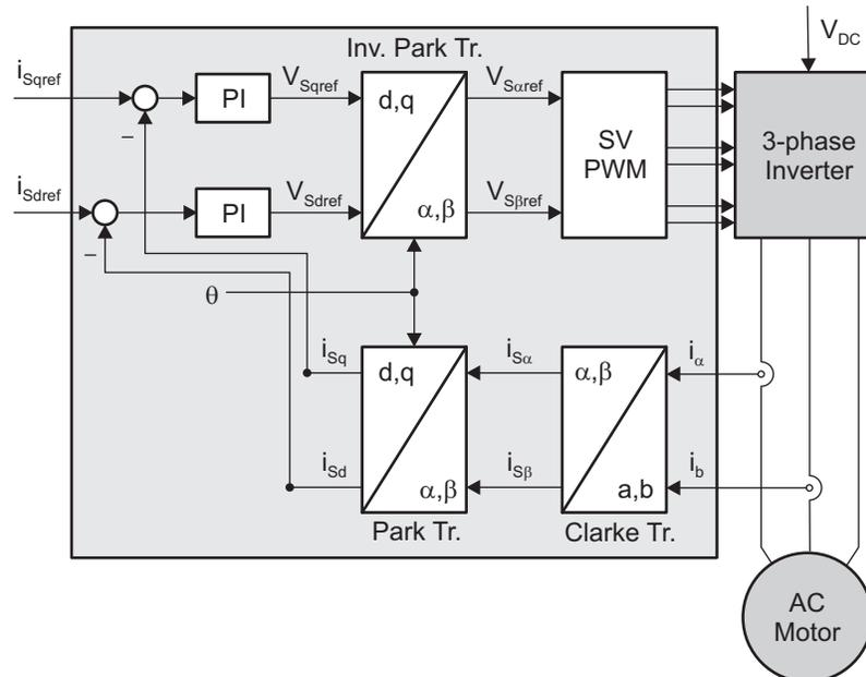
**Figure 1. Basic Scheme of FOC for AC Motor**
