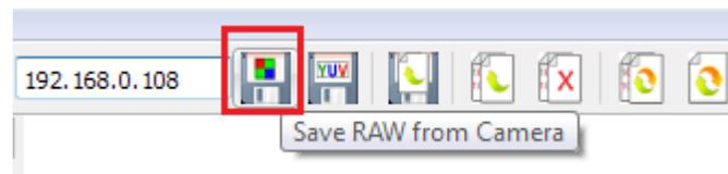
Captures a RAW frame from the sensor and allows you to save to a location on PC.
