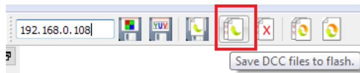
Write selected DCC files and write to QSPI Flash on the EVM. The change is persistent and will be applicable on next reboot.
