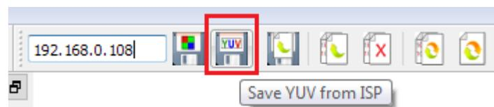
Captures a YUV frame from ISP output queue and allows you to save to a location on PCa.
