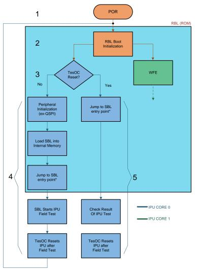
Figure 2. TDA3xx SoC IPU TESOC Boot Sequence
