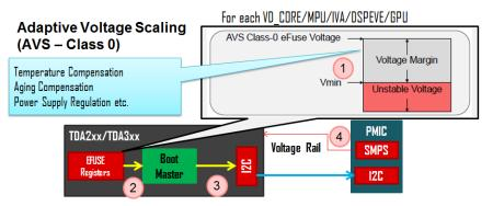
Figure 3. AVS Class 0 Voltage Scaling Mechanism
