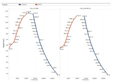
Figure 22. Thermal Tracking by Changing Thermal Thresholds in Temperature ISR
