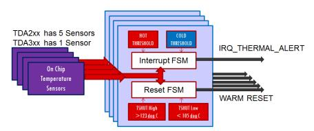
Figure 19. Functional Block Diagram of the Thermal Sensors
