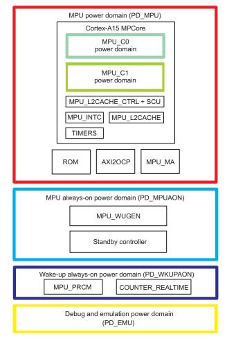
Figure 10. MPU Subsystem Power Domains
