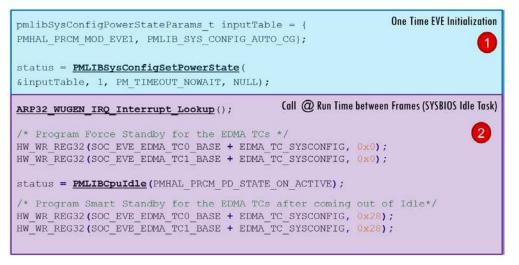
Figure 18. Recommended Software Flow for EVE to go to AUTO\_CG
