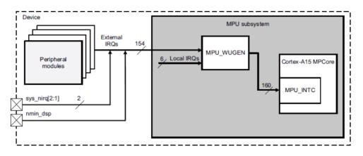
Figure 11. MPU Wake Up Generator Block in MPU Subsystem
