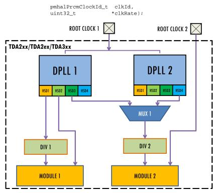
Figure 6. PRCM Representative Clock Tree Structure
