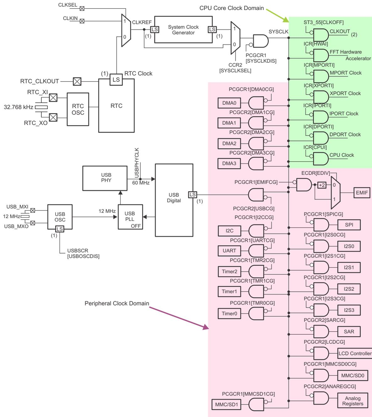
**Figure 3. C55x5 Clock Diagram**
