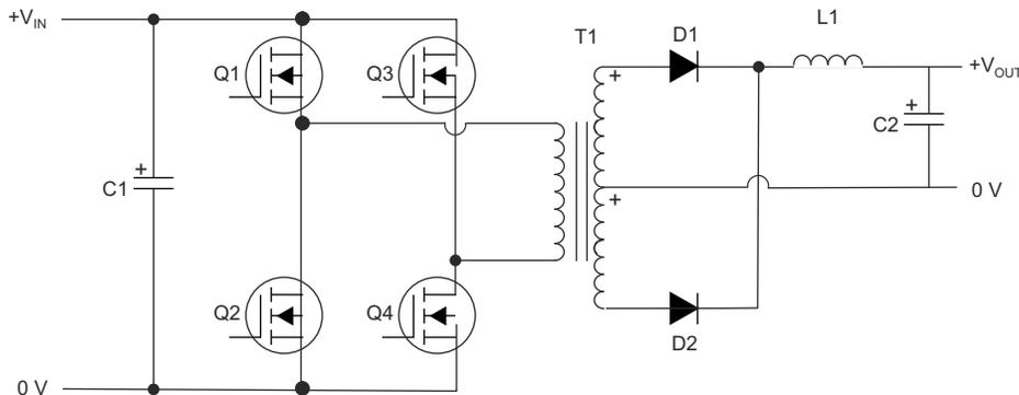
**Figure 3-3. Full Bridge Converter**
