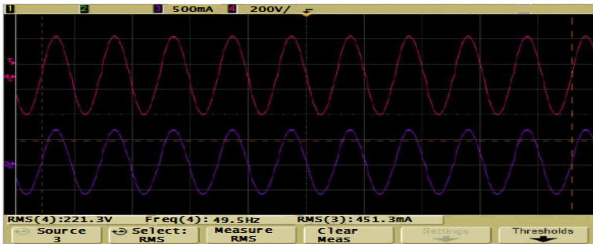
Figure 9-2. Output Voltage and Current (100W Load)
