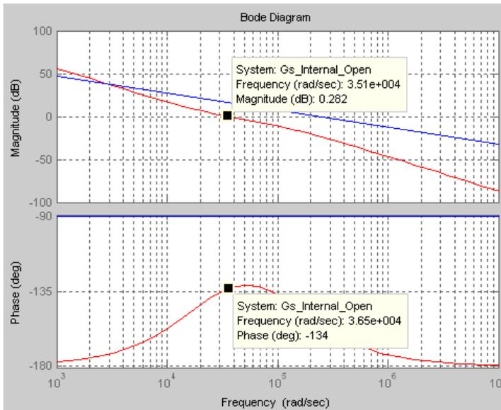
**Figure 8. Internal Open-Loop Frequency Response**
