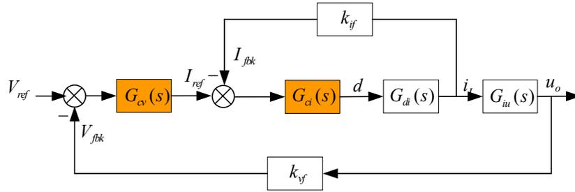
**Figure 7. Current Mode Control Block Diagram**
