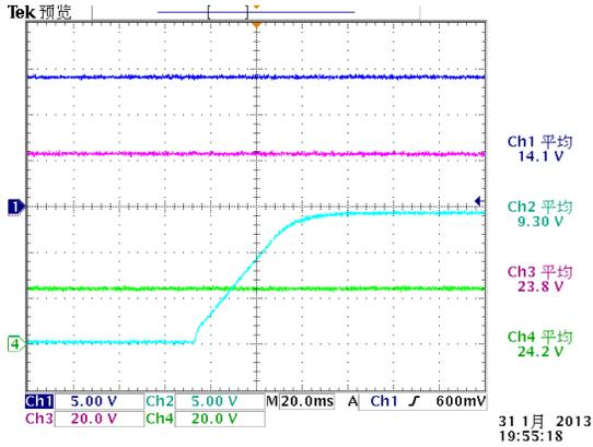
Figure 11. Buck Voltage Mode Soft Start Test
