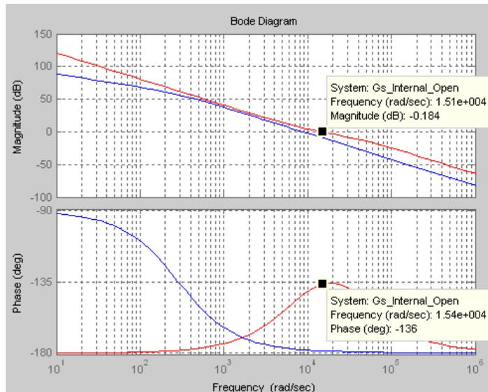
**Figure 6. Voltage Mode Open-Loop Response for Boost**
