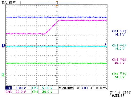
Figure 17. Boost Current Mode Soft Start Test
