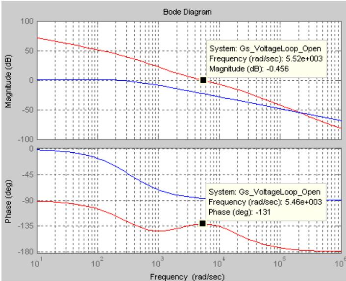
**Figure 9. External Open-Loop Frequency Response**
