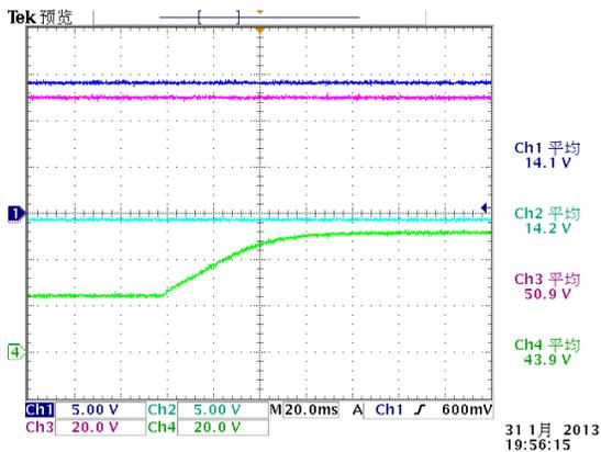
Figure 13. Boost Voltage Mode Soft Start Test
