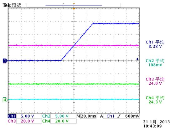
Figure 15. Buck Current Mode Soft Start Test
