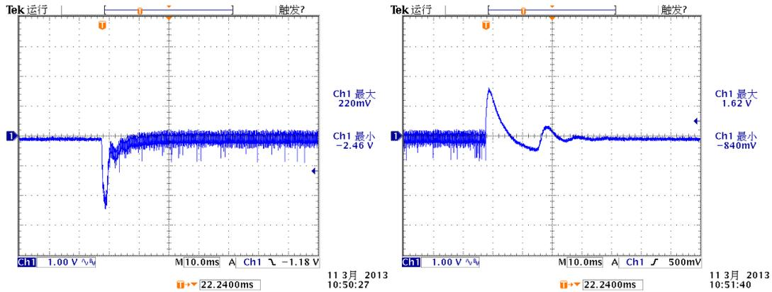
Figure 14. Boost Voltage Mode Load Step Test
