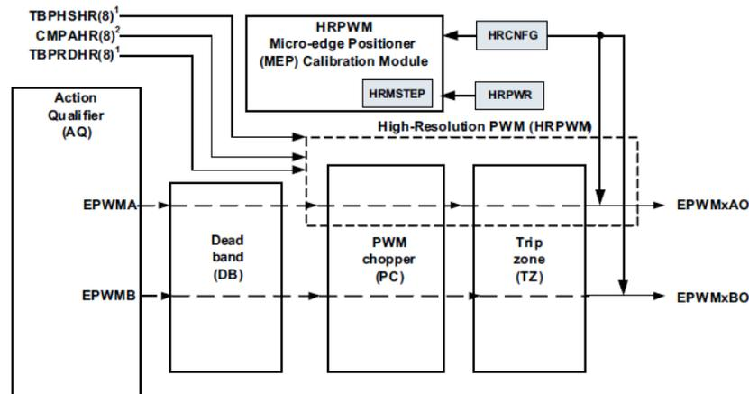
**Figure 10. The Block Diagram of HRPWM**
