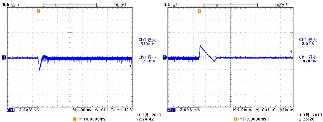
Figure 18. Boost Current Mode Load Step Test
