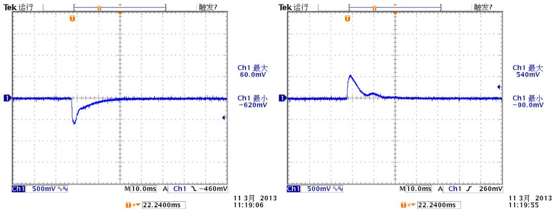
Figure 12. Buck Voltage Mode Load Step Test
