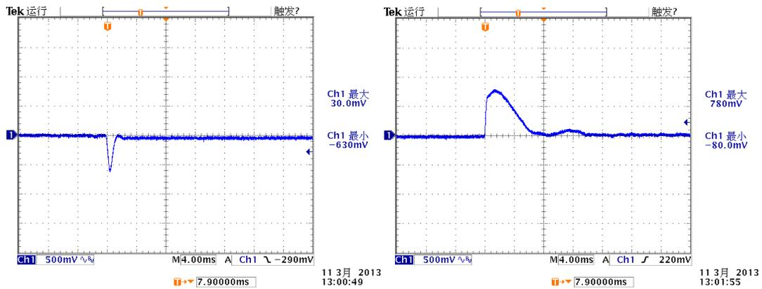
Figure 16. Buck Current Mode Load Step Test
