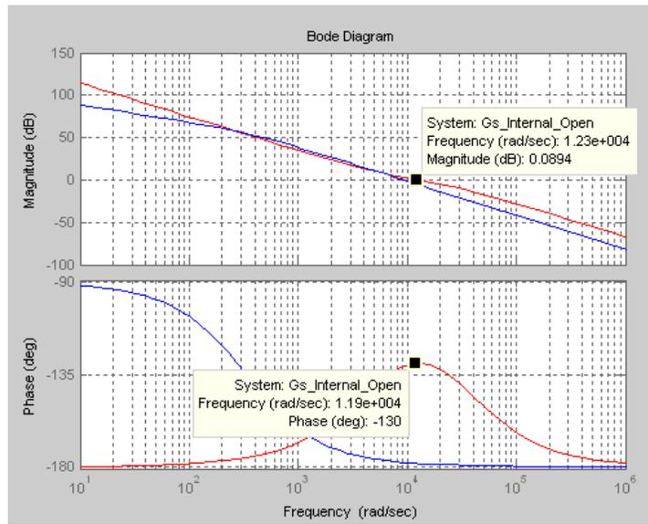
**Figure 5. Voltage Mode Open-Loop Response for Buck**
