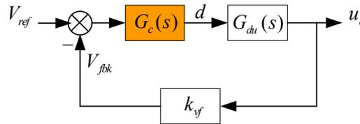
**Figure 4. The Voltage Mode Control Block Diagram**
