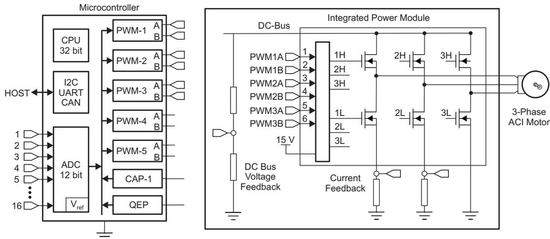
**Figure 10. A 3-ph Induction Motor Drive Implementation**
