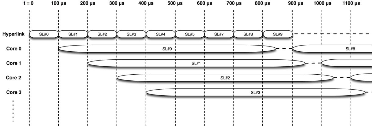
**Figure 10. Example timing diagram for input data streaming into MSMC SRAM of a DSP in case one scanline is acquired every 100  $\mu$ s and assuming that it takes 740  $\mu$ s for each core to beamform a scanline. Each core starts processing the scanline assigned to it after all the data for that scanline are transferred into MSMC SRAM. In this diagram, it is assumed that data are brought from ADCs into C6678's MSMC SRAM via Hyperlink.**
