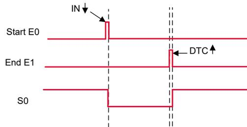
**Figure 4-2. State Machine in the FSW Block**
