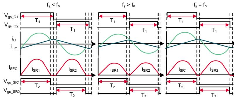
**Figure 1-1. Desired SR Driving Signal Under Different  $f_s$**
