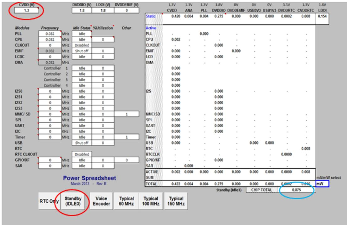
**Figure 1. IDLE3 Power Snapshot**
