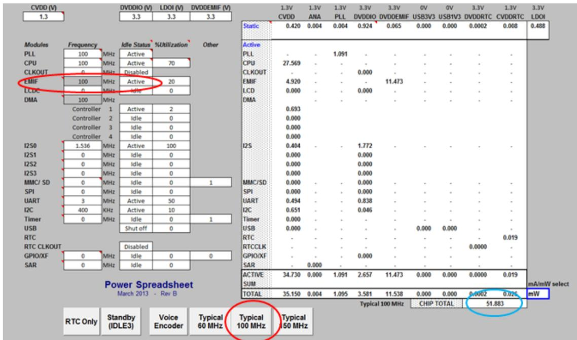
Figure 3. 100-MHz Power Calculation (with EMIF)
