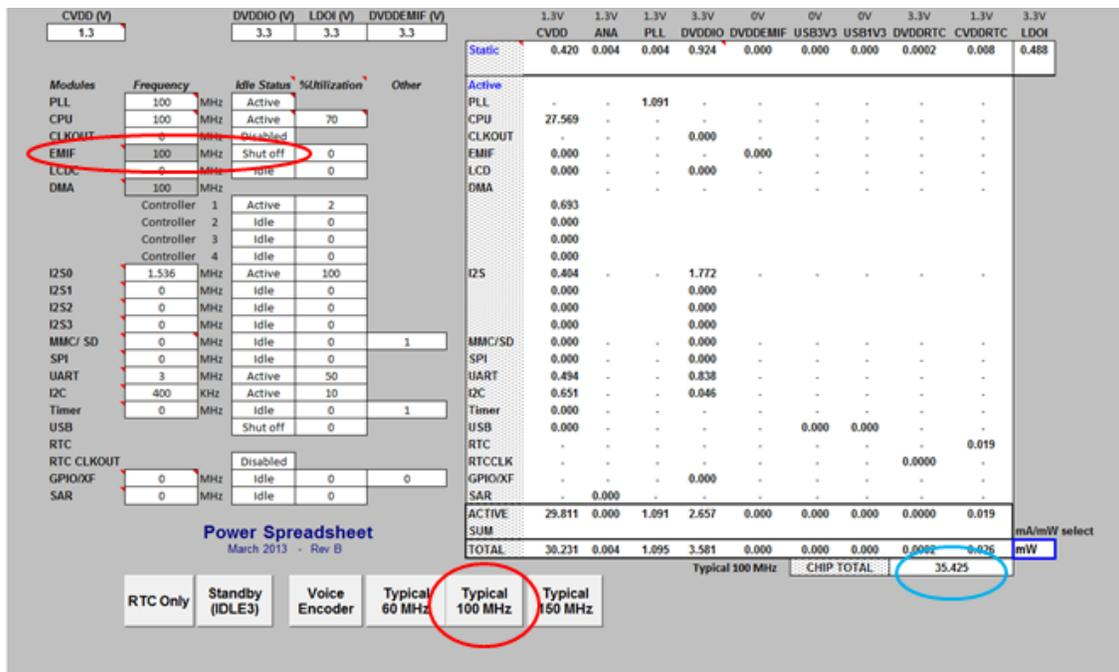
Figure 4. 100-MHz Power Calculation (with no EMIF)
