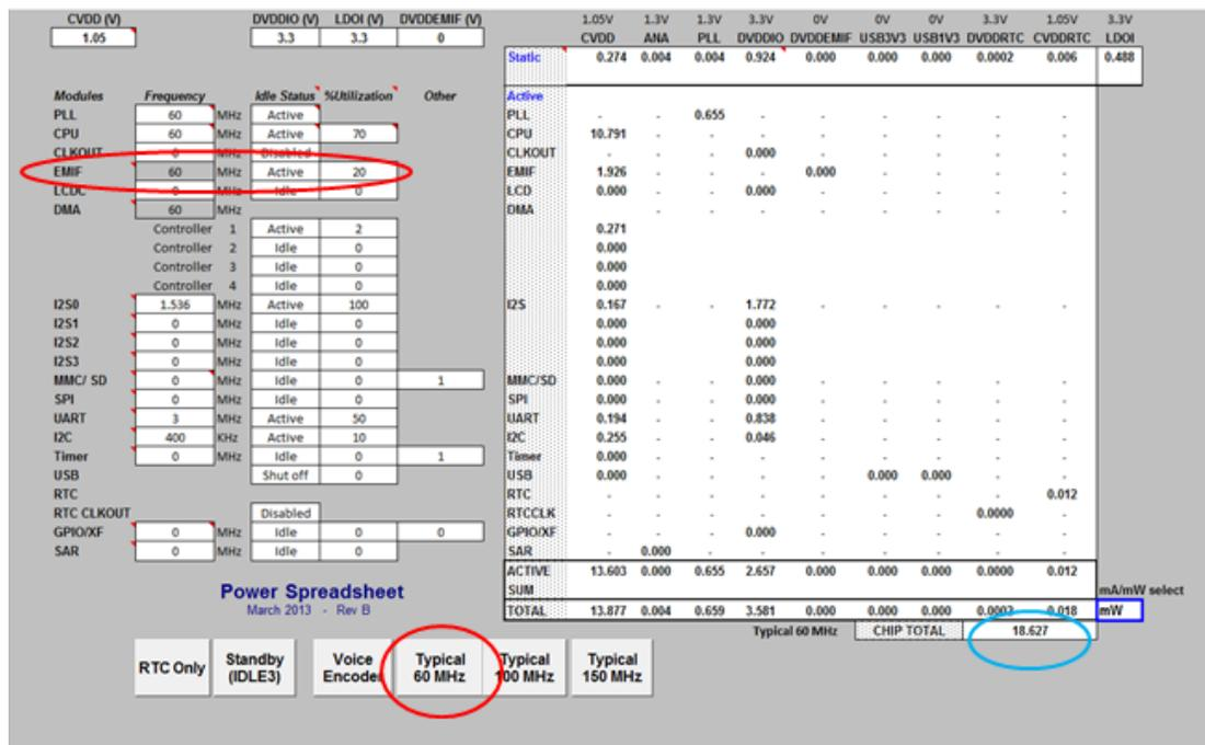
Figure 2. 60-MHz Power Calculation (with EMIF active)
