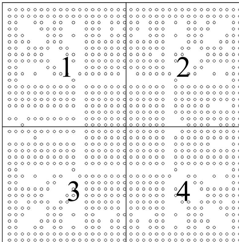
**Figure 1. DM816x Footprint With Via Channel Array**
