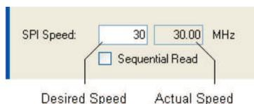
For I2C- and SPI-master modes, you can enter the desired speed. Depending on the PLL settings and granularity supported by the I2C and SPI peripherals, AISgen calculates the actual speed and shows it in an adjacent box. Recent I2C devices support speeds up to 400 kHz, and SPI devices support speeds up to 33 MHz.
