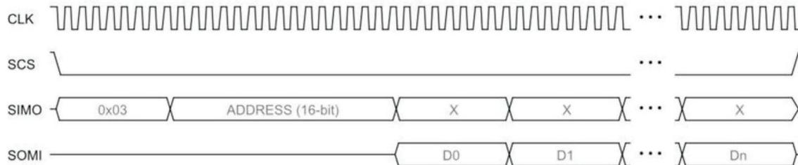
**Figure 29. SPI Signal Diagram for SPI EEPROM Boot**
