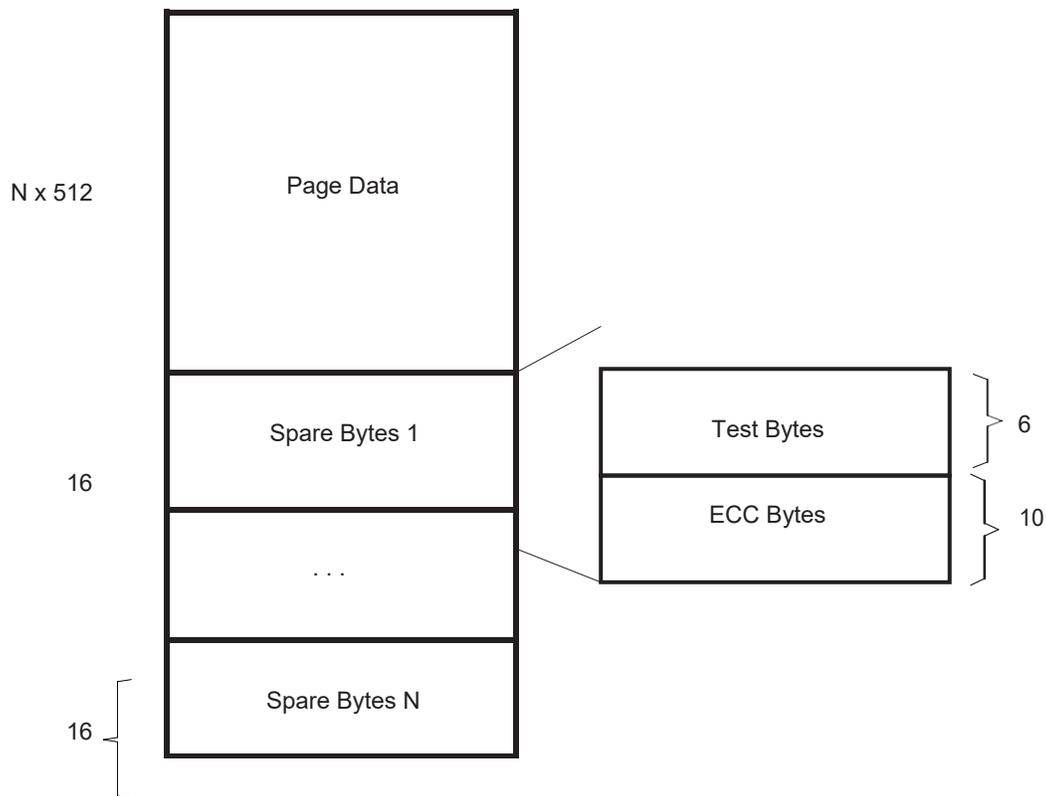
**Figure 22. Structure of NAND Page and Spare Bytes**
