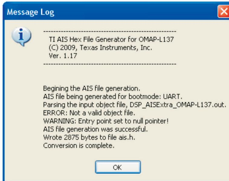
For example, the above error message indicates that the specified DSP application executable file is not in TI COFF format and AISgen failed to parse it.
