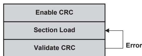
For slave-boot modes, the external master reads the calculated CRC from the device and validates it against the expected value from AIS. In case of an error, it is up to the external master to decide how many times it wants to retry loading the section before reporting failure.
