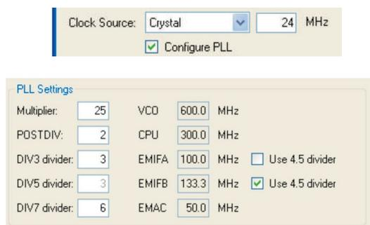
When changing any of these values, calculated frequencies will update to reflect the changes. The multiplier and divider values that you have to enter are the actual multiplication and division factors (x), not the values that get programmed into the corresponding PLL registers (x - 1). The default settings of the PLL dividers that are not configurable are shown in [Table 3](#).
