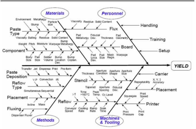
Figure 12. Fishbone Diagram Highlighting Various Causes and Effects Surrounding Assembly Yield
