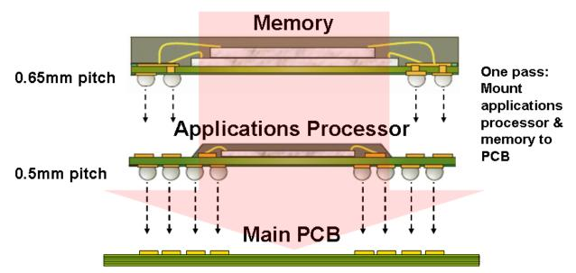
Figure 3. One-Pass Assembly
