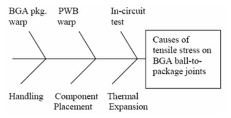
Figure 11. Causes of Stress on BGA Packages and Solder Joints
