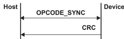
**Figure 12. Validate CRC Flow for Slave Mode**
