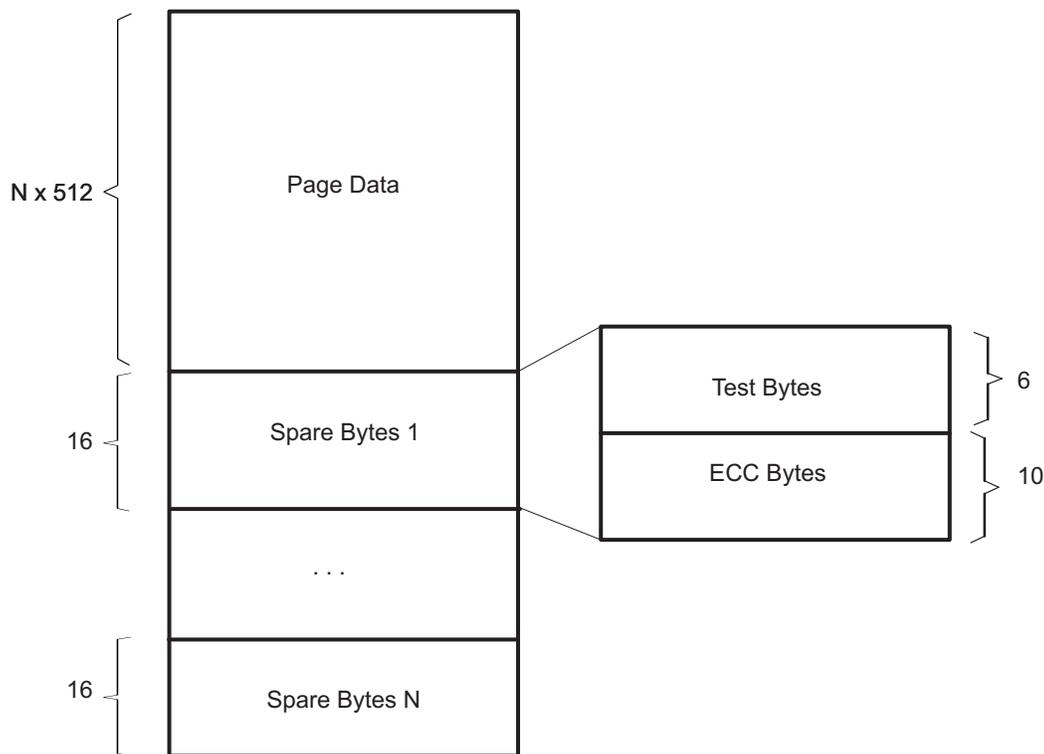
**Figure 21. Structure of NAND Page and Spare Bytes**
