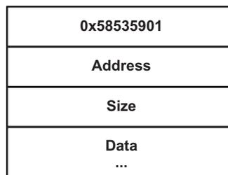
Figure 6. Section Load Command
