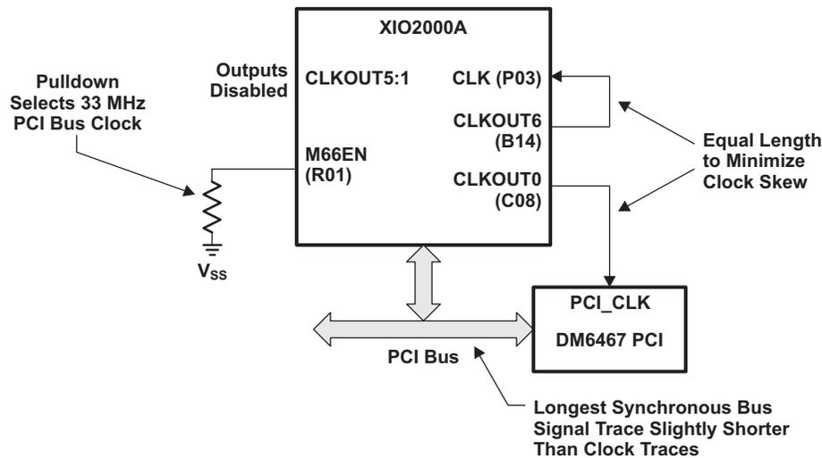
Figure 5. External PCI Bus Clock Feedback
