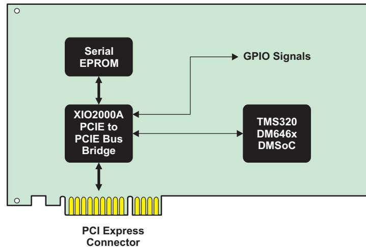
**Figure 3. Bridge Adaptor Card Block Diagram**
