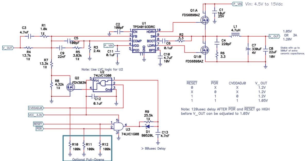
Figure 6. SR Power Supply Reference Design With Pulse Gating (Core)
