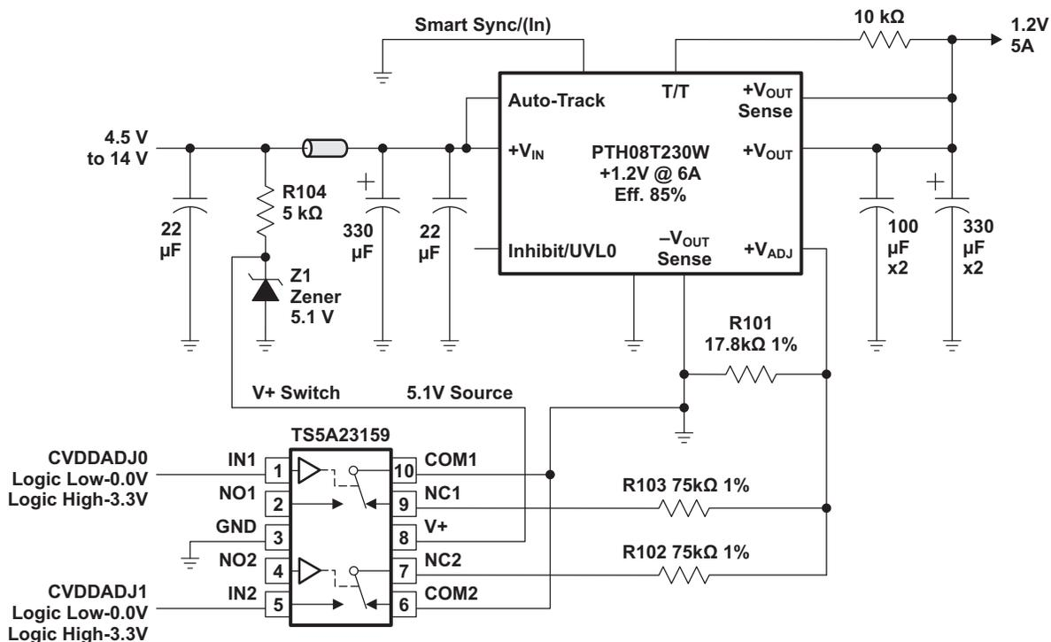
Figure 4. SR Power Supply Reference Design (Core)
