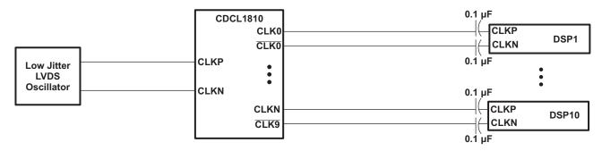
Figure 9. Multiple Devices 1.8 V LVDS Clock Solution
