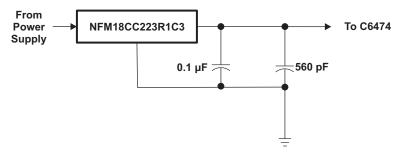
Figure 13. Recommended Power Supply Filter
