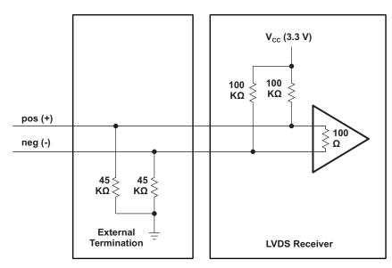
Figure 30. External Terminations: Receiver With 100  $\boldsymbol{\Omega}$
