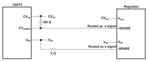
Figure 16. Single DSP Remote Sense Connections
