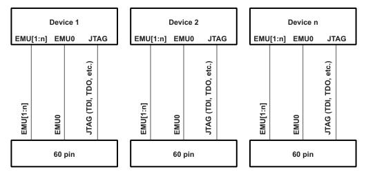
Figure 22. Emulator With Trace, Solution #1
