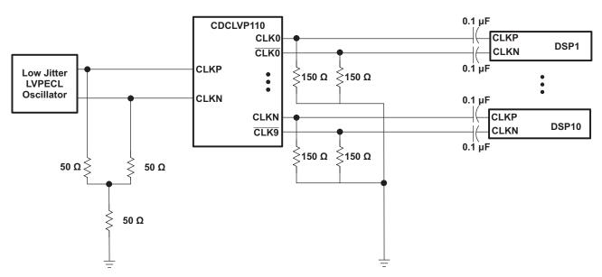
Figure 8. RIOCLK Multiple Devices LVPECL Clock Solution
