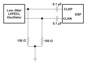
Figure 5. Differential Single Device LVPECL Clock Solution
