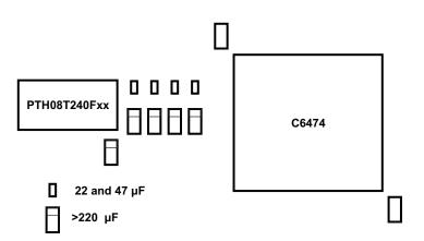
Figure 17. Bulk Capacitor Placement
