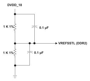
Figure 14. V<sub>REFSSTL</sub> Reference Voltage
