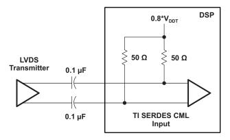
Figure 26. LVDS to CML Connection
