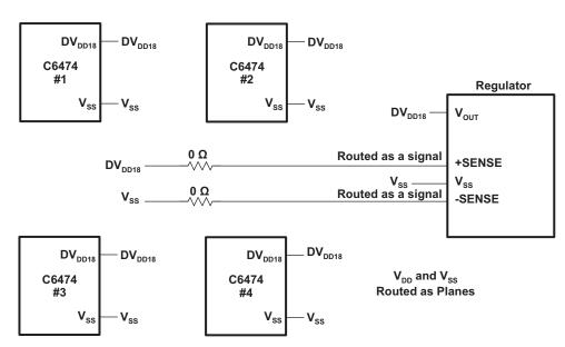
Figure 15. Multiple DSP Remote Sense Connections
