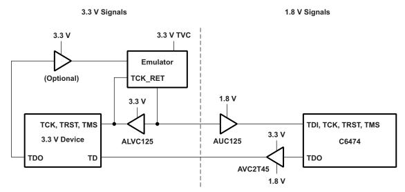
Figure 24. Emulator Voltage Translation With Buffers
