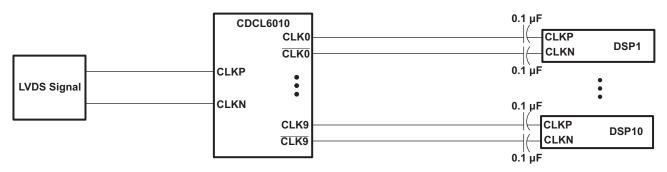
Figure 10. CDCL6010 Solution With LVDS Input
