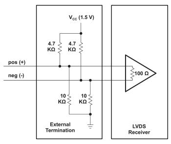
Figure 29. External Terminations: Receiver With 100  $\Omega$
