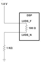
Figure 21. Unused LVDS Connections
