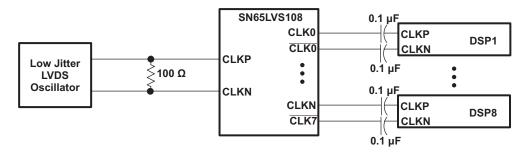
Figure 7. Multiple Devices LVDS Clock Solution
