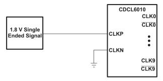
Figure 11. CDCL6010 With Single Ended Input
