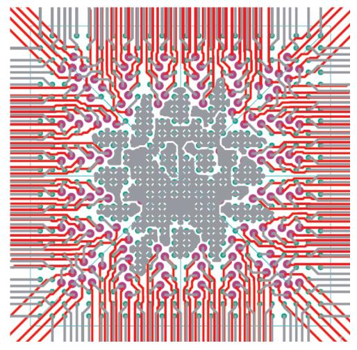
Figure 6. Completed Layout in Two Signal Layers (four overall layers)
