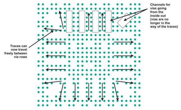
Figure 1. OMAP35x Footprint With Via Channel Array
