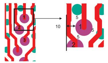
A This illustration shows an even closer look at the number 1 and 2 vias on the right of the illustration. The places where the number "5" appear show the distance from the number 1 via to the surrounding area in mils (5 mils = 0.125mm). It also shows how the number 2 via is placed as close as possible to the number 1 via, but offset by 10 mils (.250mm).
