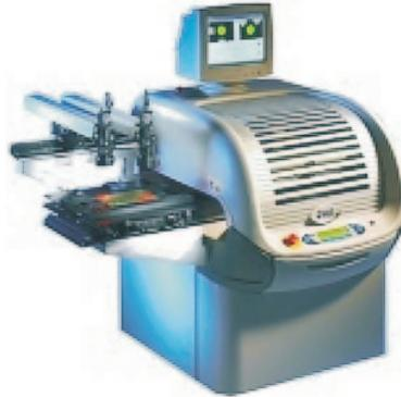
**Figure 9. DEK 248 Screen Printer**
