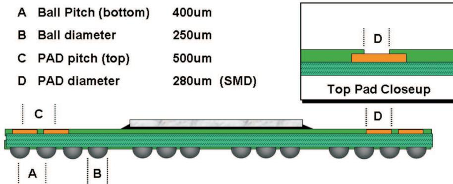
Figure 5. OMAP35x - CBB Package Specification Details
