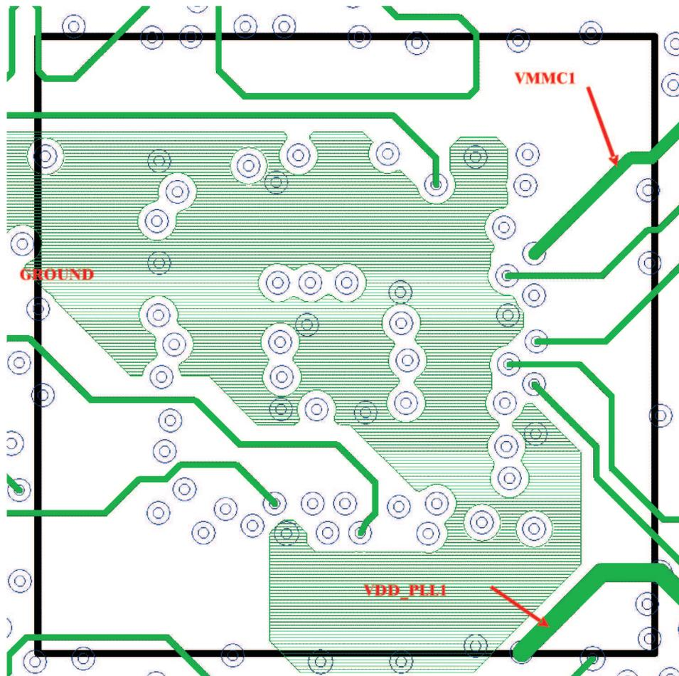
Figure 22. Close-Up of BeagleBoard Layer 4 - Internal Signal
