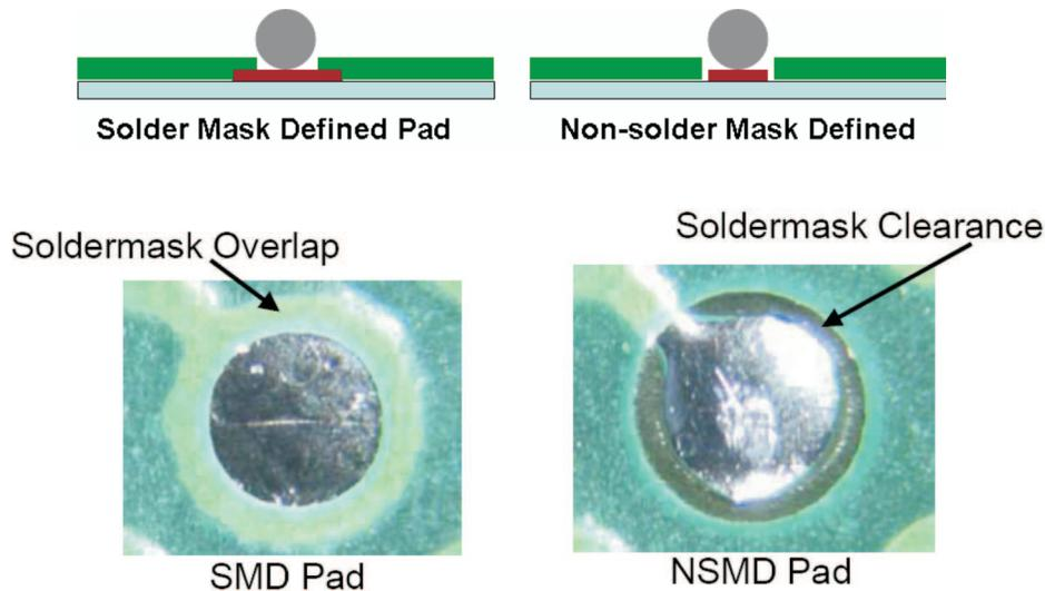
**Figure 7. Solder-Mask-Defined (SMD) and Non-Solder-Mask-Defined (NSMD) Pads**
