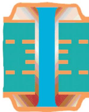
**Figure 14. Plated, Filled and Capped BGA Pad**
