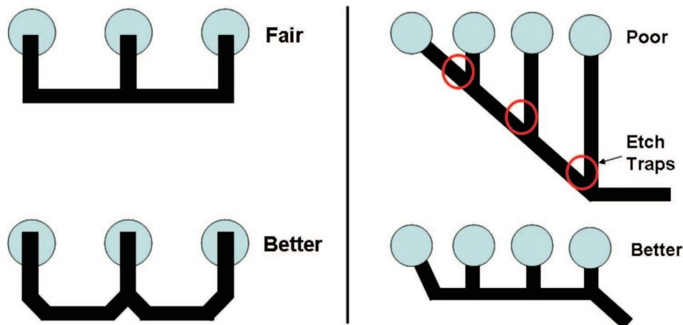
**Figure 11. Common Sense Routing Circuit Board Guidelines**
