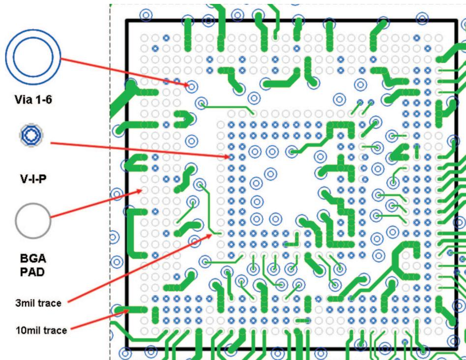
Figure 18. BeagleBoard Top Layer Underneath the OMAP35x
