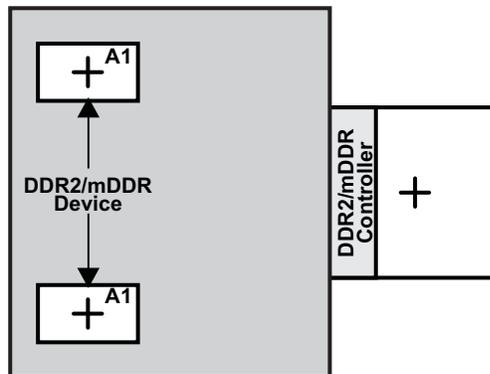
Region should encompass all DDR2/mDDR circuitry and varies depending on placement. Non-DDR2/mDDR signals should not be routed on the DDR signal layers within the DDR2/mDDR keep out region. Non-DDR2/mDDR signals may be routed in the region provided they are routed on layers separated from DDR2/mDDR signal layers by a ground layer. No breaks should be allowed in the reference ground layers in this region. In addition, the 1.8 V power plane should cover the entire keep out region.
