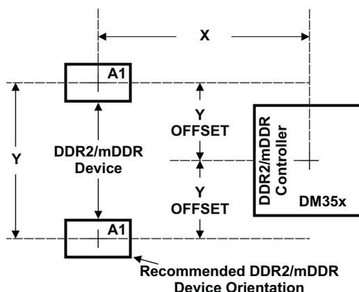
**Figure 3. DM35x and DDR2/mDDR Device Placement**
