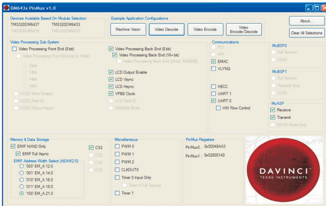
Figure 3. Video Decode Configuration
