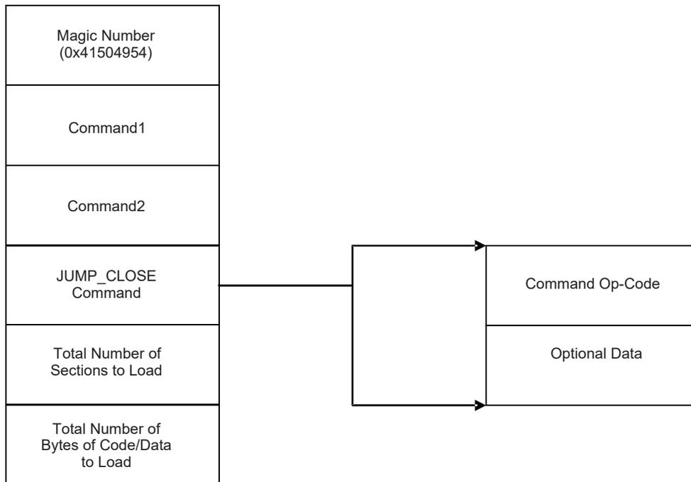
Figure 5. Basic Structure of Application Image Script
