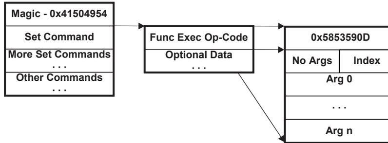
Figure 15. Structure of Function Execute Command
