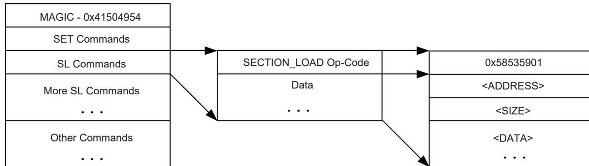
**Figure 9. Structure of Section Load Command**
