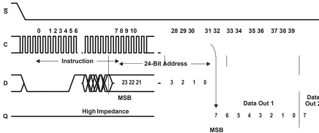
**Figure 3. 24x8 Bit SPI EEPROM Read Timing**
