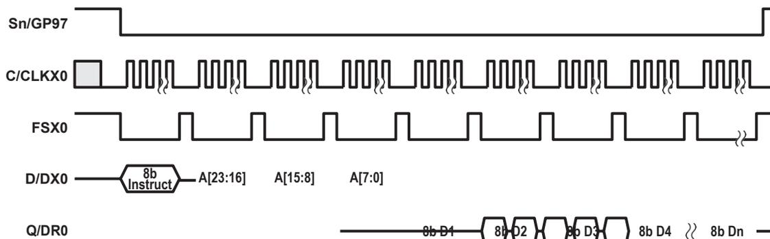
**Figure 4. DM643x 24x8 Bit Address SPI Boot**
