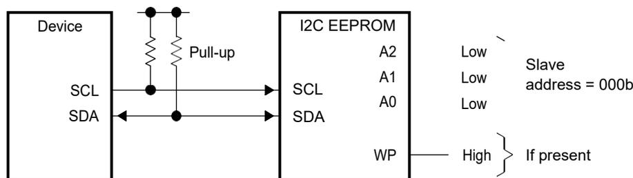
Figure 1. Signal Connections for I2C EEPROM Boot Mode
