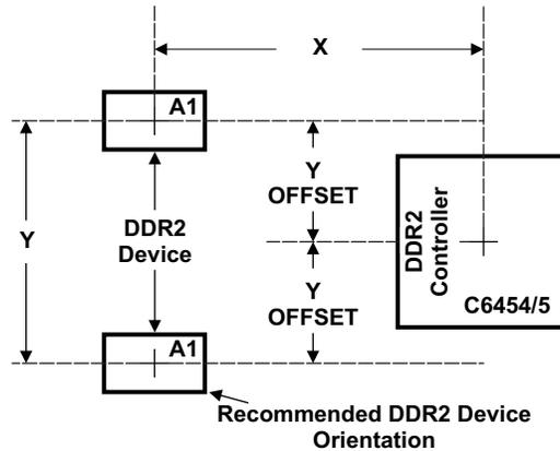
**Figure 3. C6454/5 and DDR2 Device Placement**
