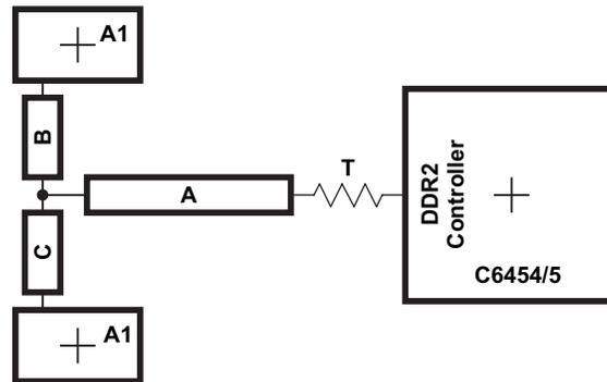
Figure 6. CK and ADDR\_CTRL Routing and Topology
