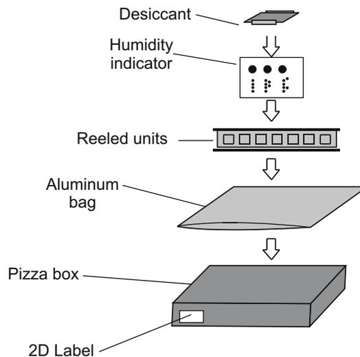
**Figure 5-5. Tape-and-Reel Packing**
