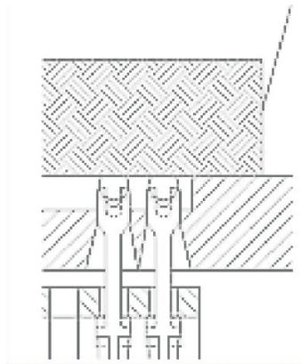
**Figure 6-6. Micro Tuning Fork Contact for 0.5mm Pitch**
