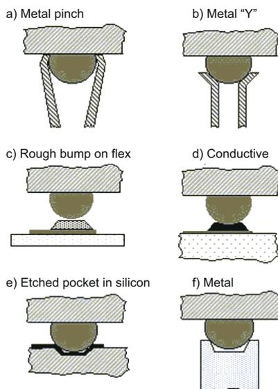
**Figure 6-1. Approaches for Contacting the Solder Ball**
