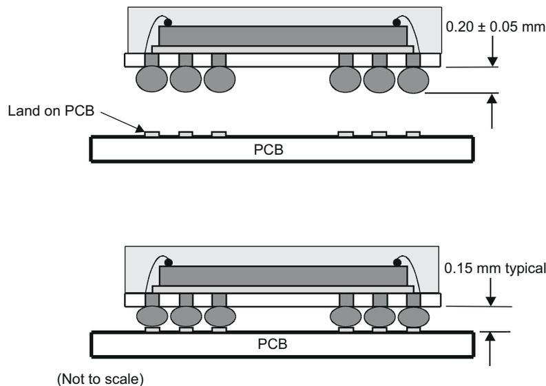
**Figure 4-1. Solder Ball Collapse**
