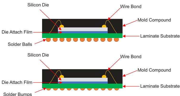
**Figure 1-3. Structure of TI's Small Body nFBGA Packages**
