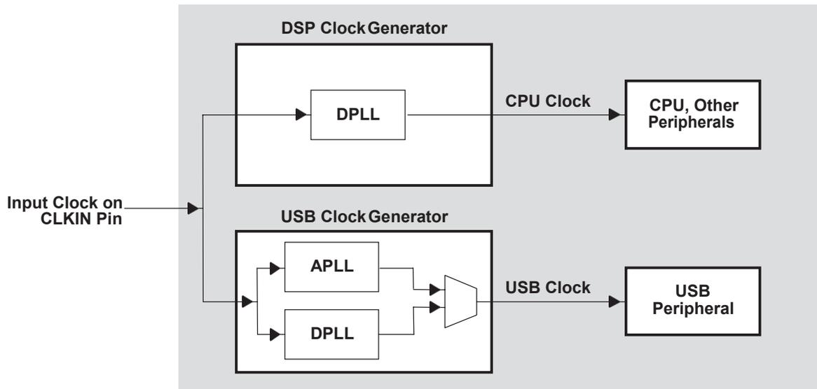
**Figure 1. High-Level View of C5506/C5507/C5509A Clocking Architecture**
