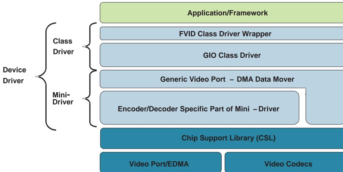
**Figure 2. DM642 Video Capture and Display Driver Architecture**
