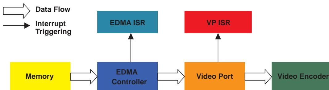
**Figure 3. Block Diagram of the Display Driver**
