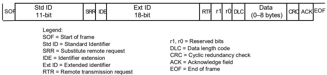
**Figure 1. Data Frame (With Extended Identifier)**
