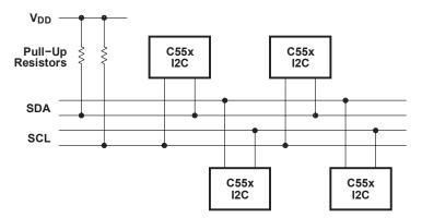
Figure 1. Multiple C55x I2C Connections
