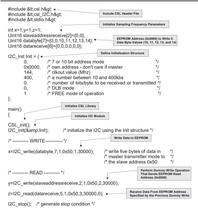
Figure 5. EEPROM Read/Write Example Code
