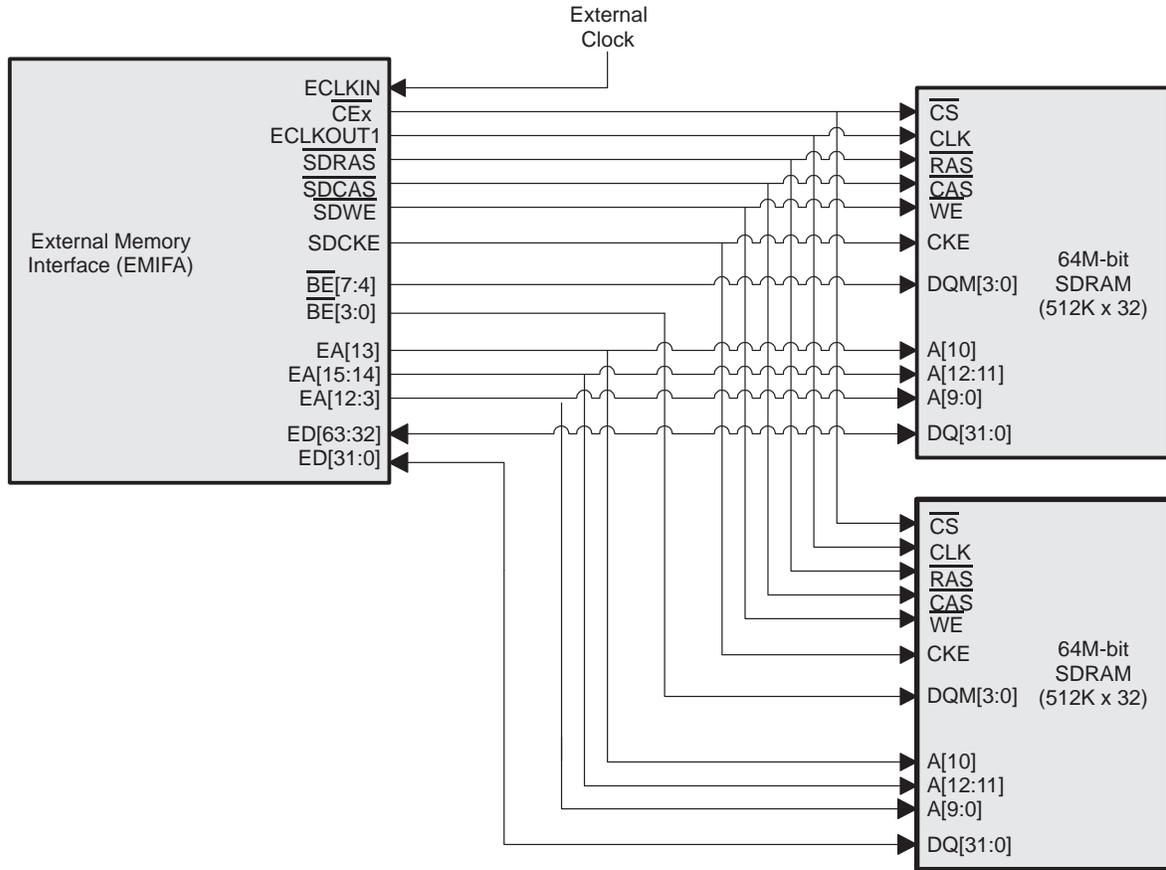
Figure 6. C64x EMIFA-to64M-Bit SDRAM Interface Using Two 32-Bit-Wide Chips
