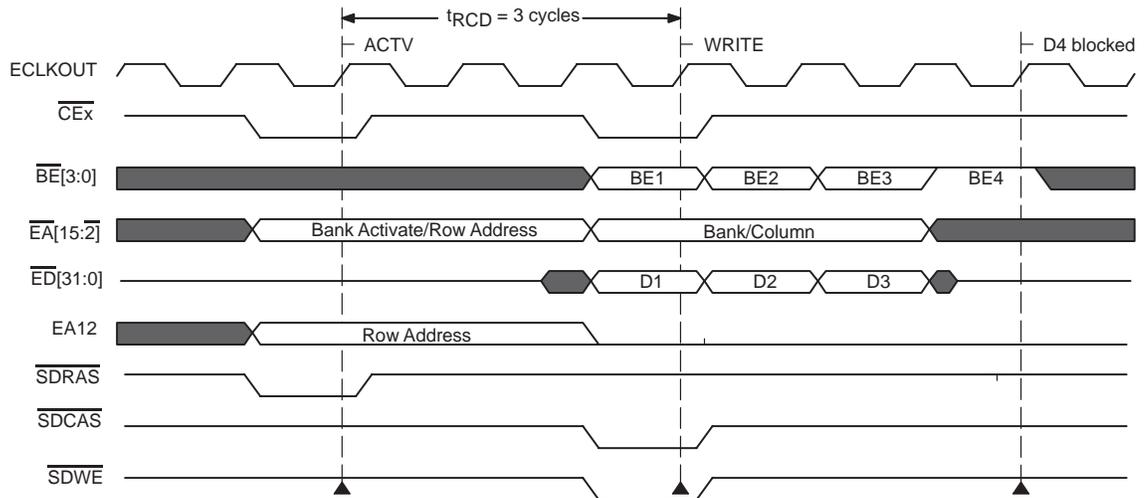
Figure 35. C621x/C671x SDRAM Burst Length 4 Write
