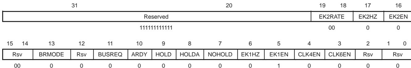
Figure 52. EMIF Global Control Register Diagram for C6414 MT48LC4M32B2
