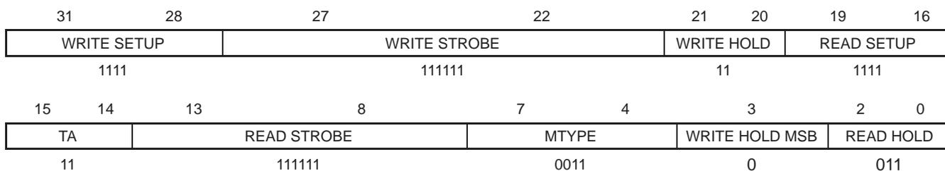
Figure 53. EMIF CE2 Space Control Register Diagram
