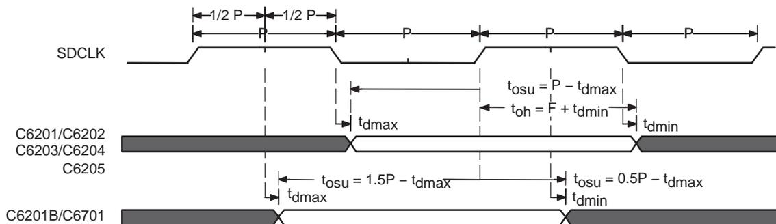
Figure 14. C6201/C6202/C6203/C6204/C6205 vs. C6201B/C6701 Output Timing
