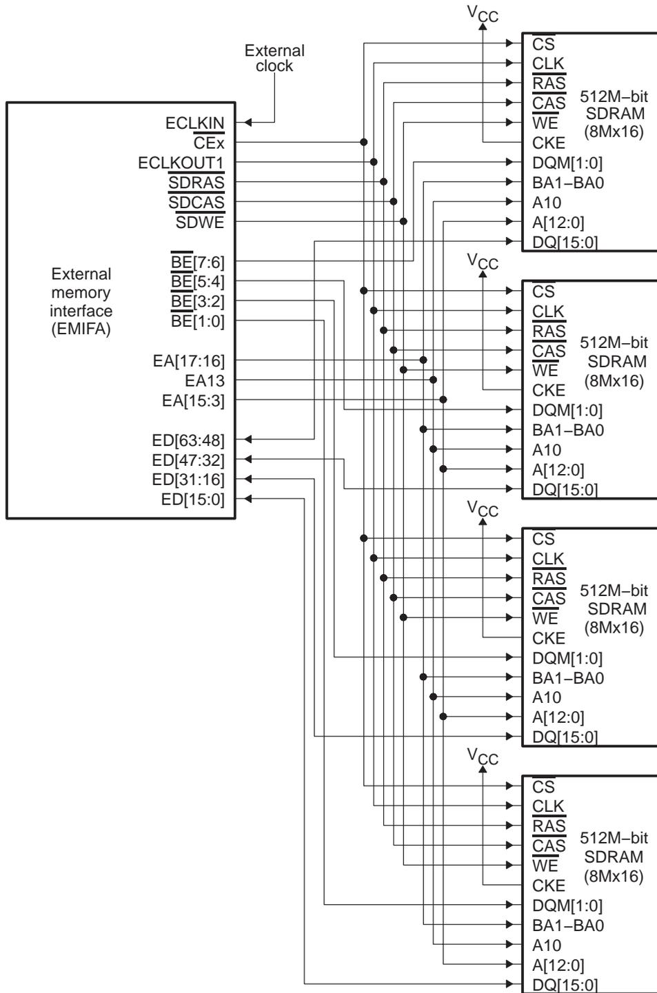
Figure 7. C64x EMIFA-to-512M Bit SDRAM Interface Using Four 16-bit Wide Chips
