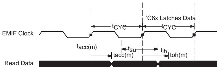
Figure 43. Input to C6000 (Read Data)
