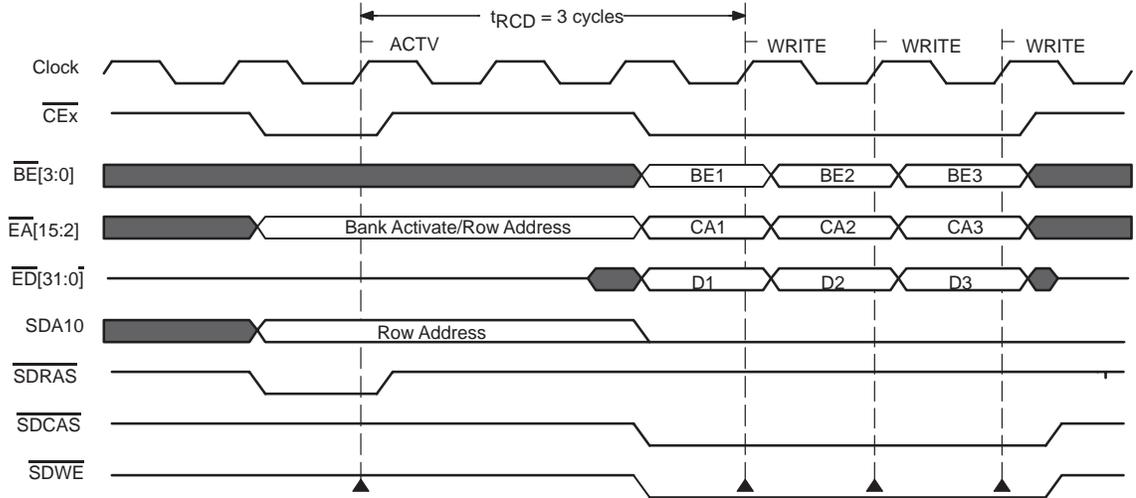
Figure 34. C620x/C670x SDRAM Burst Length 1 Write
