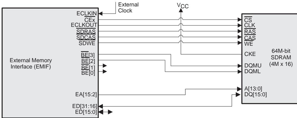
**Figure 5. C621x/C671x EMIF-to-64M-Bit SDRAM Interface Using One 16-Bit-Wide Chip (Big Endian)**
