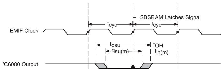
Figure 41. Outputs From C620x/C670x (Write Data [ED], Control, and Address Signals)
