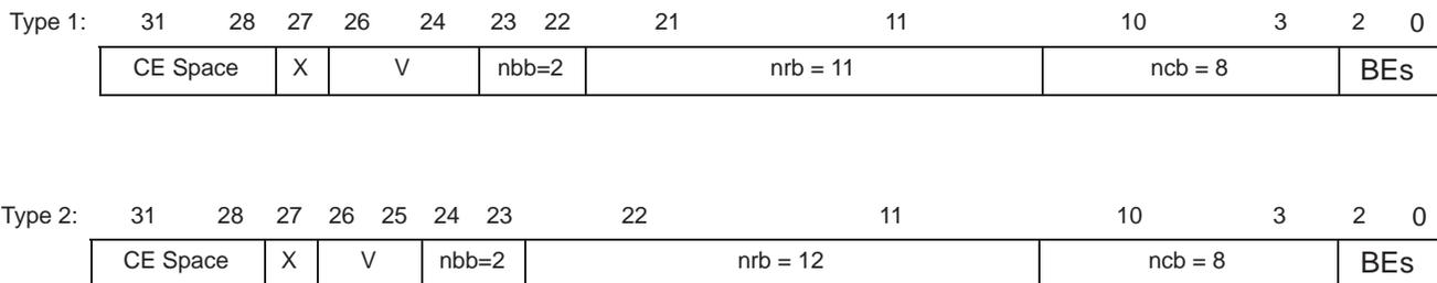
**Figure 24. SDRAM Logical Address Bits**
