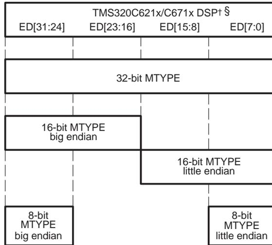
§ The C6713B and C6711D devices allow the flexibility of changing the EMIF data placement on the EMIF bus. See the device specific data sheet for more details.
