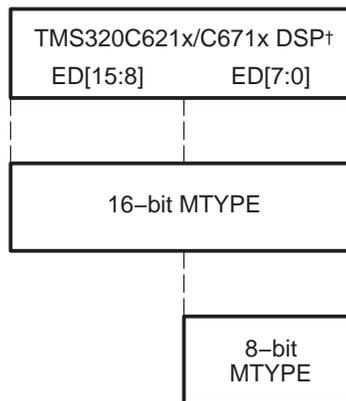
† C6712/C6712C DSP do not support big-endian byte alignment. C6712D supports both big-endian and little endian with the above data alignment. For more details, see the device specific datasheet.
