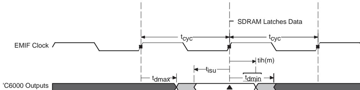
**Figure 42. Outputs From C621x/C671x/C64x (Write Data [ED], Control, and Address Signals)**
