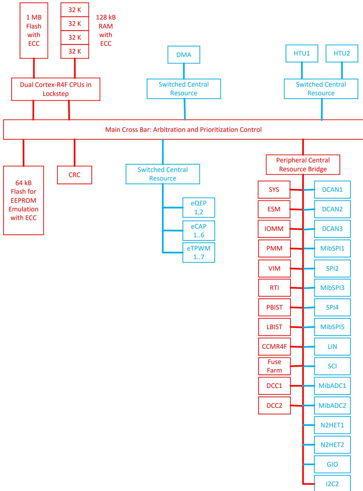
Figure 5. Partition of Hercules MCU for Safety Analysis
