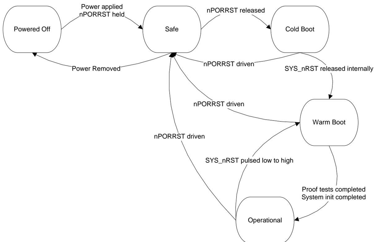
**Figure 6. Operating States of the Hercules MCU**
