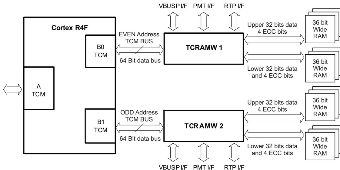
Figure 9. Block Level Implementation of CPU SRAM
