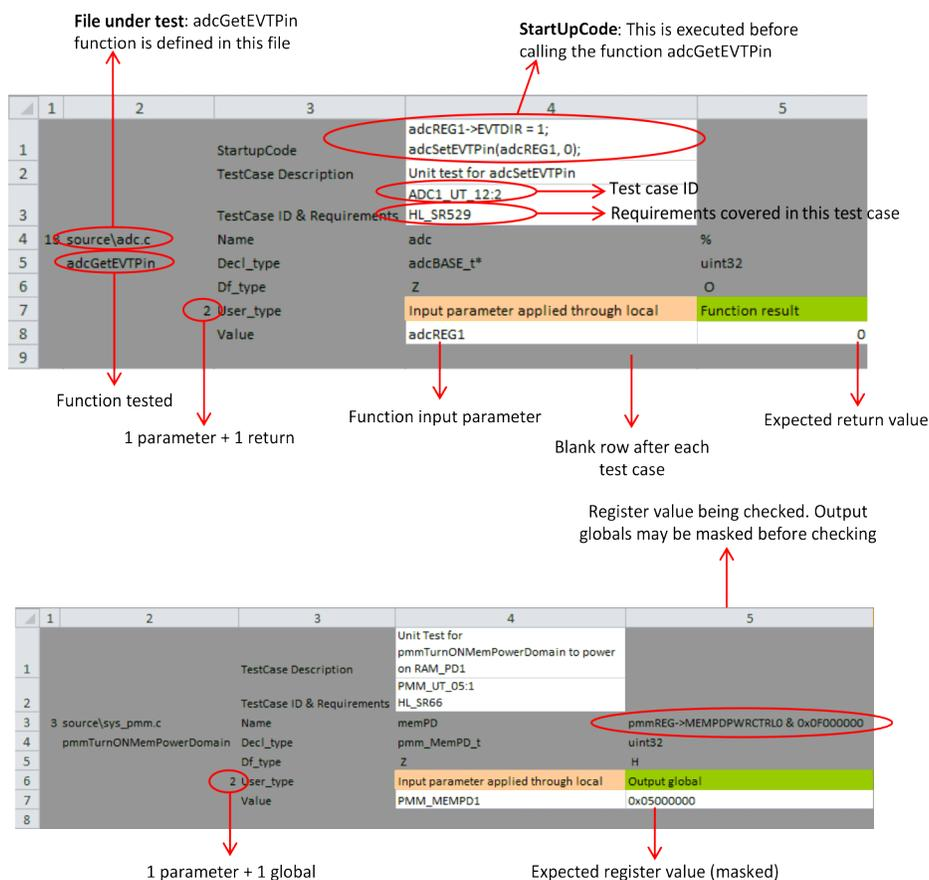
Figure 16. Examples of a Test Case
