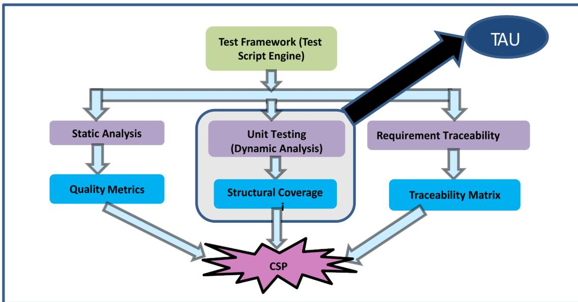
Figure 3. Test Automation Framework for CSP
