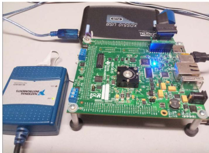
**Figure 2. Hardware Setup**
