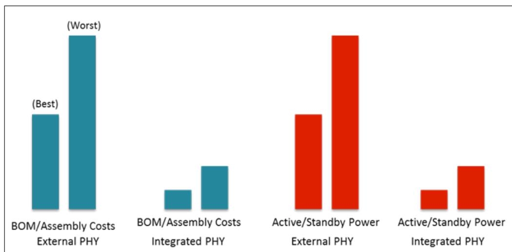
Figure 2: Significant cost, power and board space savings can be achieved when the Ethernet PHY is integrated onto the MCU as opposed to a traditional Ethernet implementation using an external PHY.
