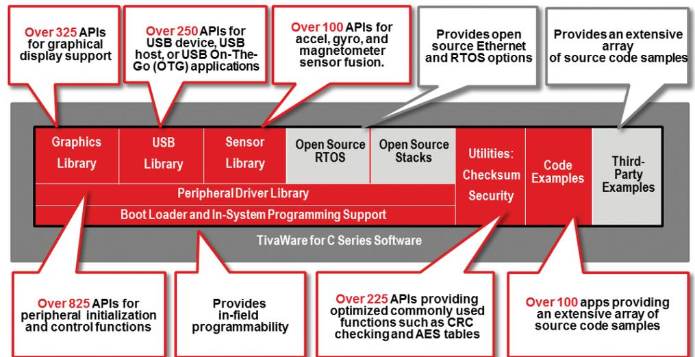
Figure 5. TI provides a wide range of low-level support firmware and libraries — including peripheral, graphics, USB and sensors — to accelerate design, increase overall system reliability and reduce development costs
