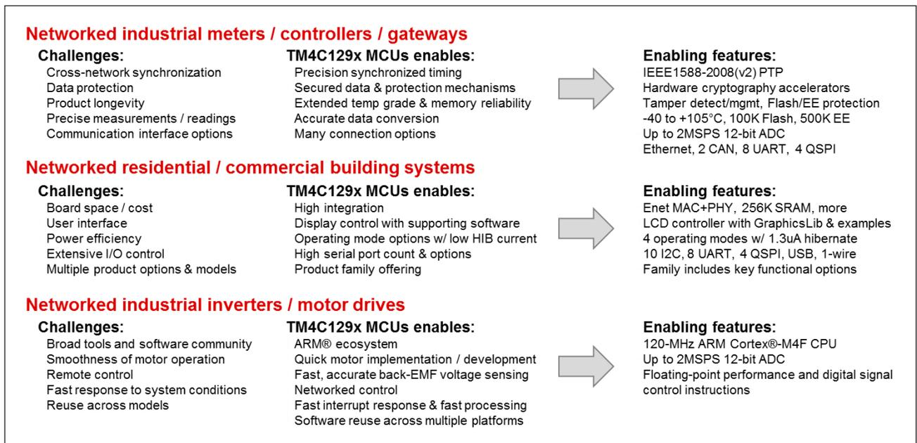
Figure 4. The advantages of the TM4C129x MCU go far beyond just the PHY savings it offers. Its architecture has been designed to address the design challenges typical of many IoT applications along with many others.
