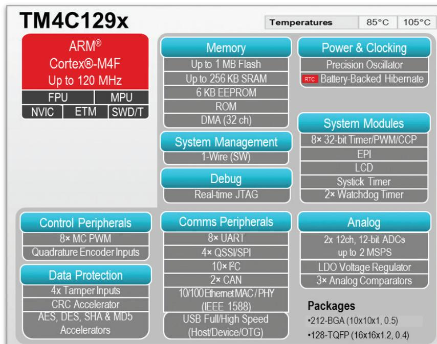
Figure 3: As the industry's first ARM Cortex-M4 MCU with integrated 10/100 MAC/PHY, TI's TM4C129x MCU has the performance, capabilities and peripherals needed to make it ideally suited for a wide range of embedded applications.
