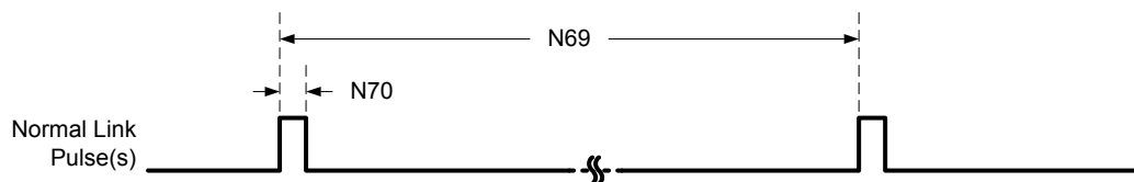
Figure 27-38. 10Base-TX Normal Link Pulse Timing
