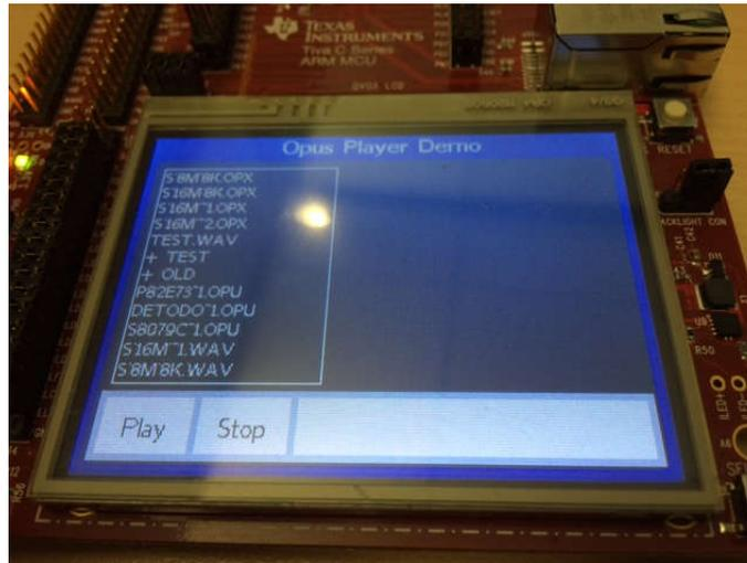
**Figure 4-7. Application opus\_playaudio\_ogg as Seen on the LCD Panel**
