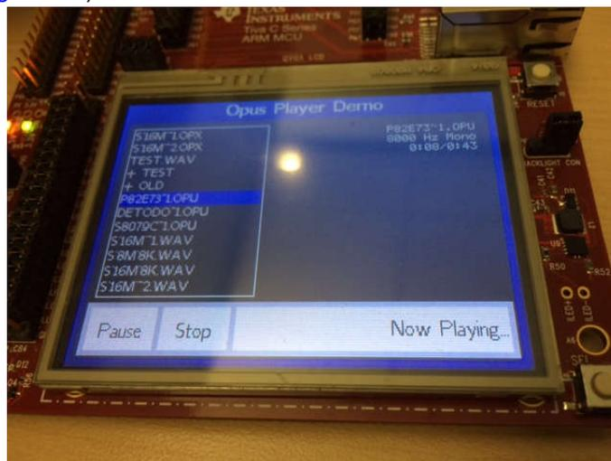
**Figure 4-8. Application opus\_playaudio\_ogg Running the Decoder**
