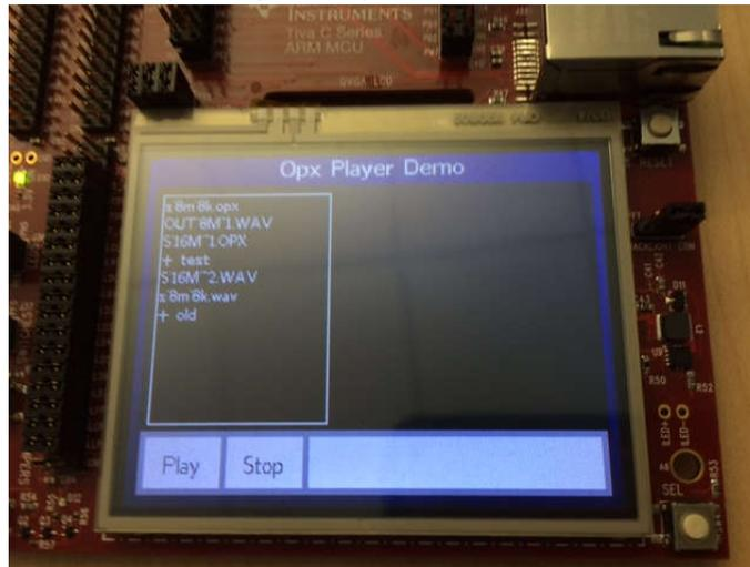
**Figure 4-5. Application opus\_playaudio\_opx as Seen on the LCD Panel**
