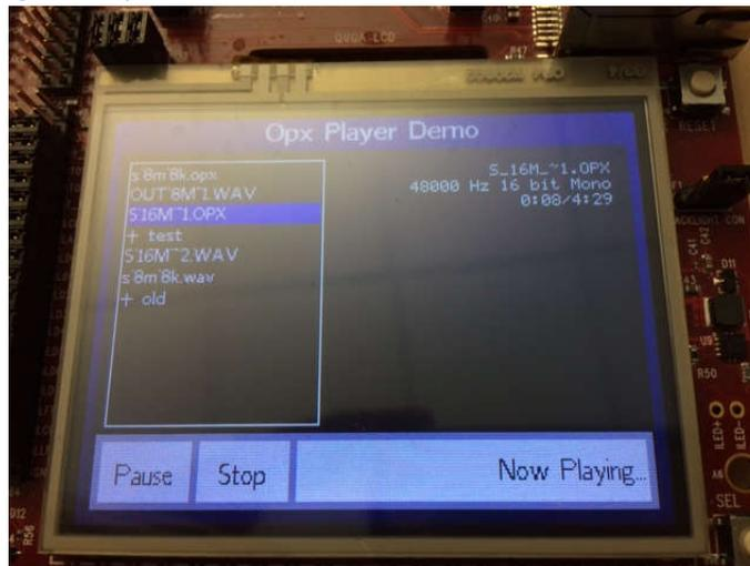
**Figure 4-6. Application opus\_playaudio\_opx Running the Decoder**
