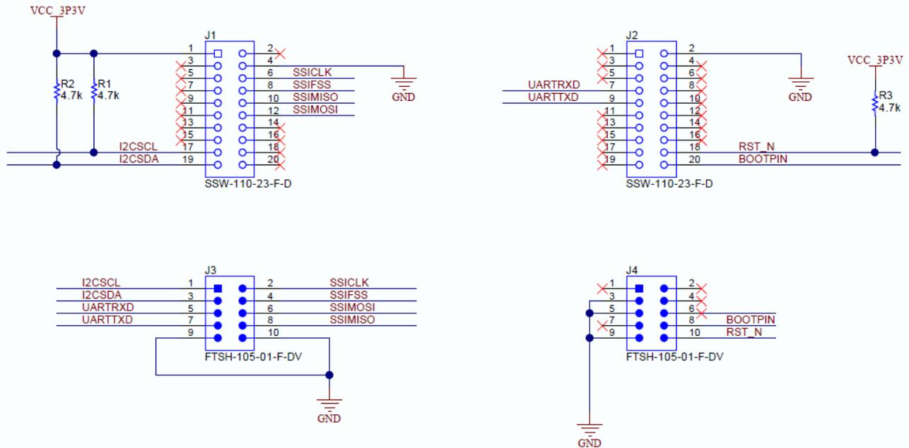
Figure 18. Schematic of EK-TM4C123GXL Connector Board
