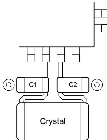
Figure 24. Recommended Layout for Small Surface-Mount Crystal
