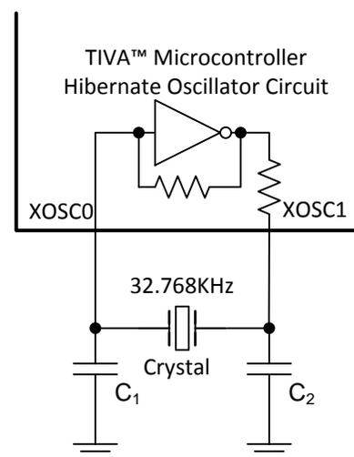
Figure 23. Hibernate Oscillator Circuit without GNDX
