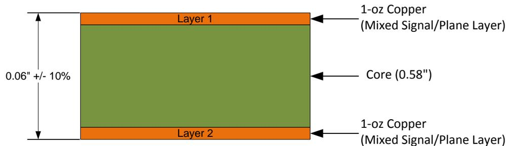
**Figure 5. Typical Two-Layer PCB Stack with Routing Assignments**
