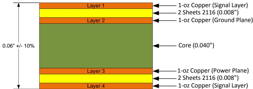
**Figure 4. Typical Four-Layer PCB Stack with Routing Assignments**
