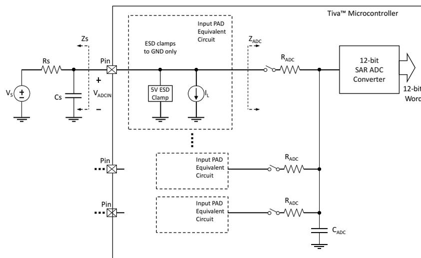
Figure 34. Tiva™ Microcontroller ADC Input Equivalency Diagram
