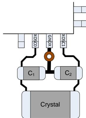
Figure 25. Recommended Layout for Crystal with GNDX Connection
