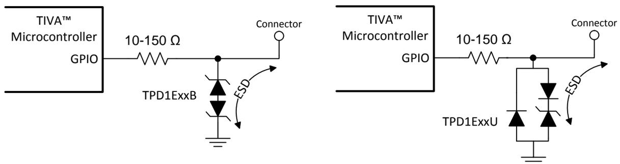
**Figure 27. General Protection Using Bi-direction TVS Diode**     **Figure 28. General ESD Protection Using Uni-direction TVS Diode**
