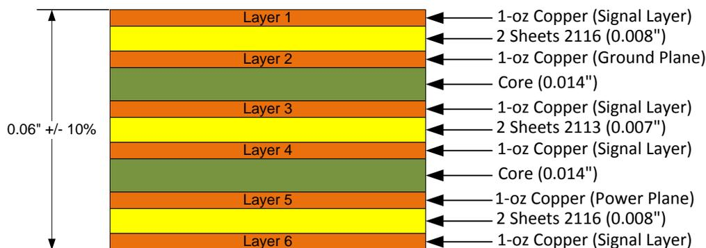
**Figure 6. Typical Six-Layer PCB Stack with Routing Assignments**
