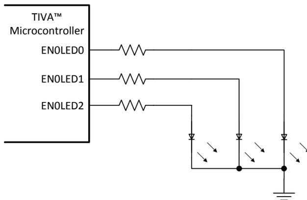
Figure 30. GPIO Sourcing LED Current
