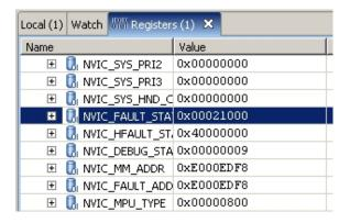
The **NVIC\_FAULT\_STAT** register has a value of 0x0002.1000, which indicates both a usage fault and a bus fault. The usage fault status bit INVSTATE is set, which means that the processor encountered a state error when it tried to execute an instruction.
