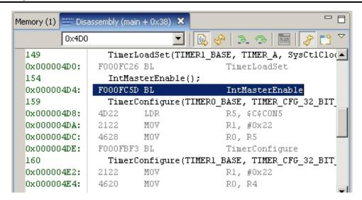
The instruction that is pointed to by the saved **PC** is a function call to <code>IntMasterEnable()</code>. However, because this is an imprecise bus fault, we know that this is not actually the instruction that caused the fault, it must be something that happened earlier in the execution. Observe that the previous instruction is another function call to the <code>TimerLoadSet()</code> function. This call is most likely where the fault occurred.
