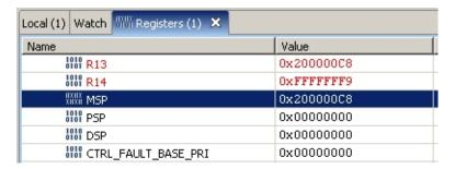
If your fault handler function has any code besides a simple infinity loop, then it may use some stack space. You must adjust the value of the stack pointer by this amount in order to find the start of the exception stack frame. For StellarisWare<sup>®</sup> examples, the fault handler function is simple and the stack pointer points directly to the exception stack frame.
