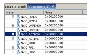
In the above screen capture, the debugger provides a view to see the value of this register. If your debugger does not provide such a view, you can examine these registers using a memory viewer starting at address 0xE000.E300. In this case, bit 19 of the first **Active Interrupt** register is set, indicating that interrupt number 19 is active and is likely the cause of the interrupt. If more than one bit is set in this register, then the highest priority interrupt is the active interrupt.
