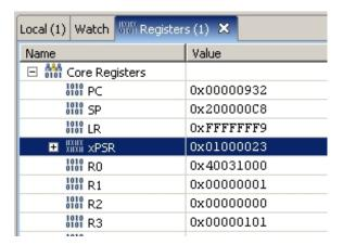
In the above example, the lower 8 bits of the **xPSR** register show the exception number is 0x23 (or 35 decimal). Referring to the Interrupts table in the "Exception Model" section of the "Cortex-M Processor" chapter of a Stellaris data sheet, shows that vector number 35 is Timer 0A.
