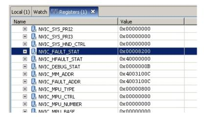
In this case, the **NVIC Fault Status (NVIC\_FAULT\_STAT)** register has a value of 0x0000.8200. Refer to any one of the documents listed in the "References" section, or to "Diagnosing Faults", to see the meaning of the bits in this register. The value shown here indicates a bus fault, and the bits that are set are BFARVALID and PRECISERR. This means that the **Bus Fault Address Register (FAULTADDR)** register contains the exact value of the address that triggered the bus fault.
