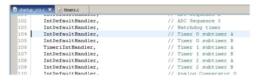
The above screen capture shows that the vector entry for Timer 0A is the IntDefaultHandler() function which is the default when no handler has been provided. In this case, the correct handler function was not entered in the table. The screen capture below shows the correct handler function entered in the vector table.
