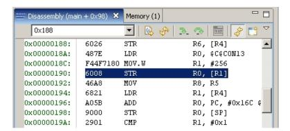
This disassembly screen capture shows that the processor was trying to execute a store (STR) instruction. It was writing the value of R1 to the location of R0. The exception stack frame shows the value of R0 was 0x0000.0100, which is the same as the value in the **MMADR**. The processor was trying to write a value to Flash memory which has been protected by the MPU.
