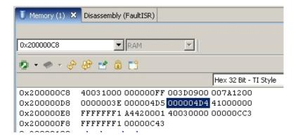
The first two rows in the screen capture above show the exception stack frame. The first row shows the saved values of registers R0-R3. The second row shows the saved value of R12, LR, PC, and **xPSR**.
