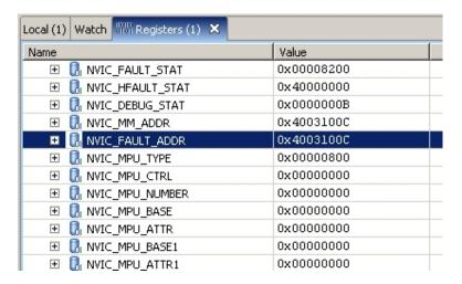
The value in the **NVIC Fault Address (NVIC\_FAULT\_ADDR)** register is 0x4003.100C. Refer to the Memory Map table in the "Memory Model" section of the "Cortex-M Processor" chapter of the Stellaris data sheet, which shows that the faulting address is in the register space of the Timer 1 peripheral.
