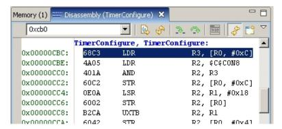
The instruction at 0x0000.0CBC is most likely the one that caused the fault. It is an LDR instruction, and is reading from the address in R0, plus an offset of 0xC. Refer back to the previous screen capture to see that the saved value of R0 was 0x4003.1000, and adding 0xC gives 0x4003.100C. The processor was trying to read from 0x4003.100C and this is likely what caused the fault. You can see that this is the same conclusion
