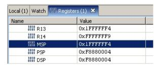
In this case, the value of the stack pointer is 0x1FFF.FFF4, which is not a valid memory location. The reason this memory location is not valid is because the stack was too small and overflowed. Because the stack overflowed, it is likely that an invalid address was used on return from a function call, and the processor **PC** was set incorrectly causing the invalid state.
