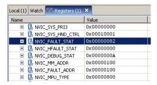
The value in the NVIC\_FAULT\_STAT register is 0x0000.0082, which means that the MMARVALID and DACCVIOL memory management status bits are set. These bits indicate that a data access violation occurred and the faulting address can be found in the Memory Management Fault Address Register (MMADR). The screen capture above also shows a value in the MMADR of 0x0000.0100, which is in Flash memory.
