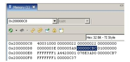
In the screen capture above, the first two rows show the exception stack frame. The first row shows the saved values of registers R0-R3. The second row begins with the saved value of R12, followed by **LR**, **PC**, and then **xPSR** register. To start with, the most interesting value is the **PC**, which is 0x0000.0CBC. There is a high probability that this points either directly at, or near the instruction that caused the fault.
