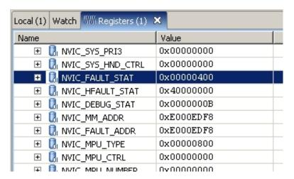
This time, the value in the **NVIC\_FAULT\_STAT** register is 0x0000.0400. The IMPRECISERR bit is set, which means that a bus fault occurred, but that the exact faulting address is not known.
