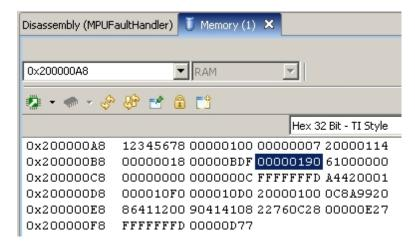
As before, the most interesting value at this point is the saved PC, which is 0x190. Disassemble the code at 0x190.
