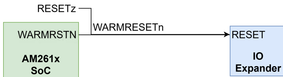
Figure 2-11. WARMRESETn Reset Signal Tree
