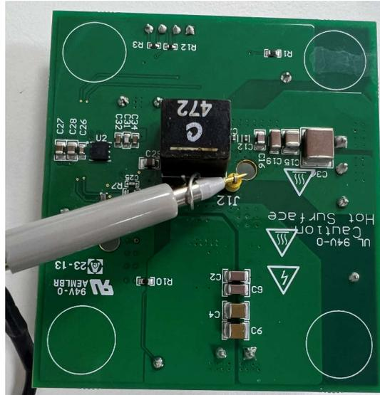
Figure 2-2. Measuring the SW Node
