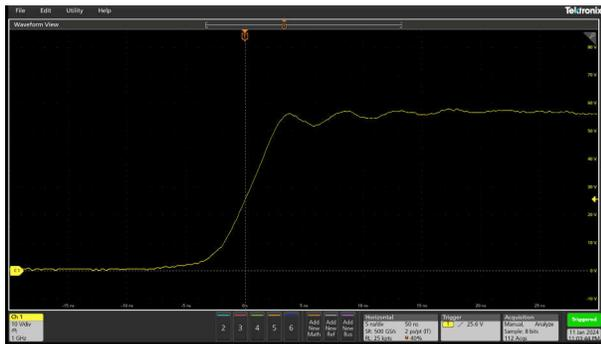
Figure 3-5. SW Node Low-Side Turn-Off
