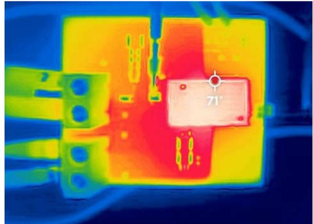
Figure 3-4. Thermal Capture of EVM After Steady State
