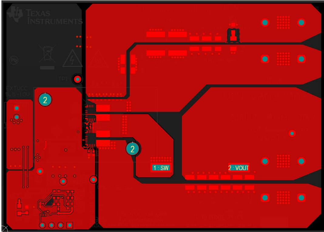
Figure 4-2. Top Layer of the PCB
