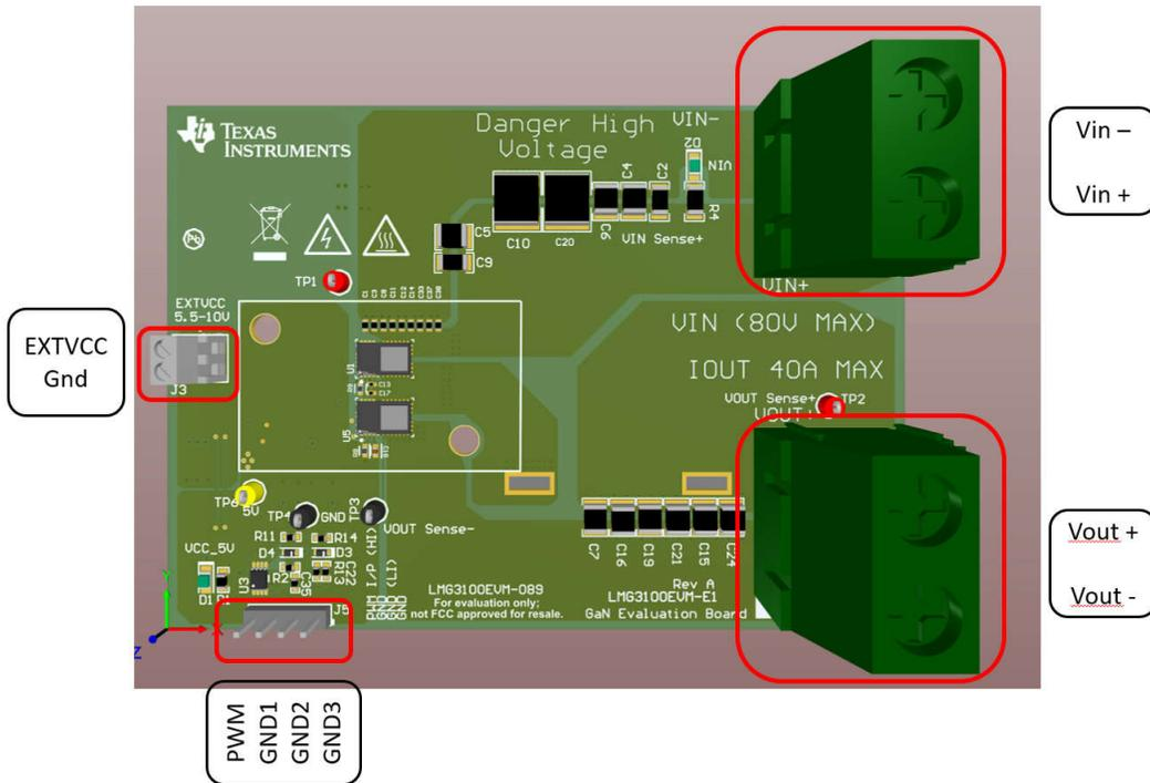
**Figure 2-1. PWM Connection on J5**
