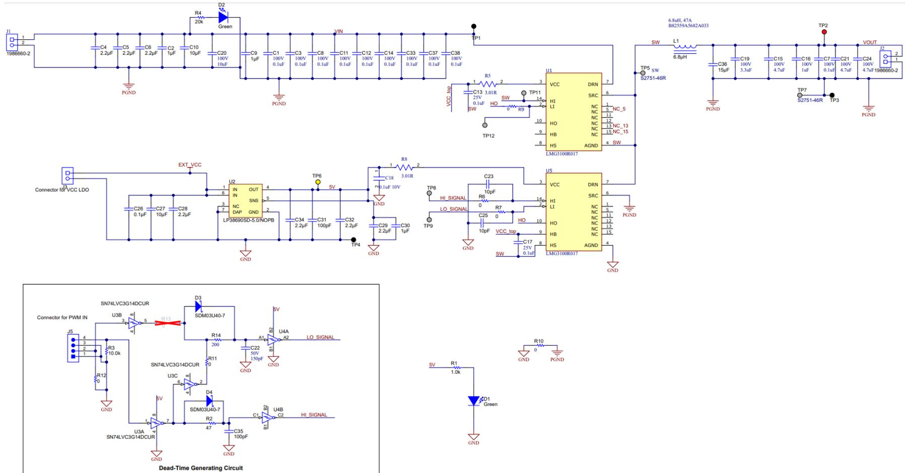
Figure 4-1. LMG3100EVM-089 Schematic
