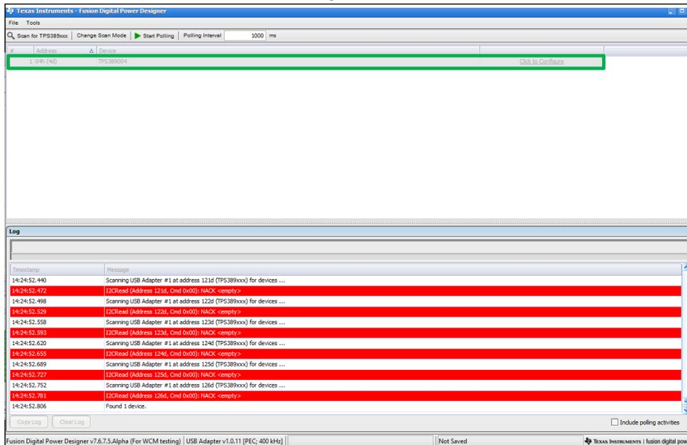
**Figure 3-11. Fusion Scan Window - Scan for TPS389C0XEVM Completed**
