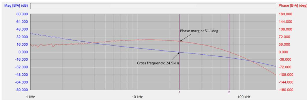
Figure 7-7. Control Loop Response:  $V_{IN} = 48\text{ V}$ ,  $V_{OUT} = 5\text{ V}$ ,  $I_{OUT} = 2.5\text{ A}$
