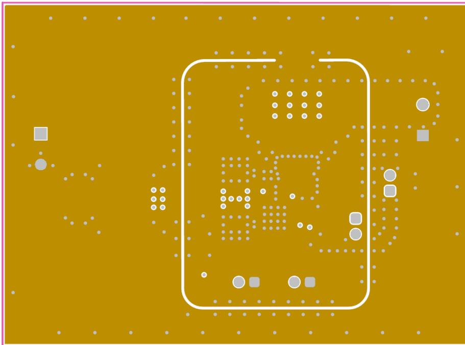
**Figure 5-2. Mid-Layer 1 Ground Plane**
