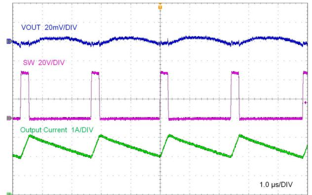
Figure 7-4. Full Load Switching:  $V_{IN} = 48\text{ V}$ ,  $V_{OUT} = 5\text{ V}$ ,  $I_{OUT} = 2.5\text{ A}$
