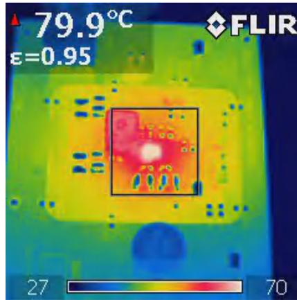
Figure 7-8. Thermal Capture of EVM:  $V_{IN} = 48\text{ V}$ ,  $V_{OUT} = 5\text{ V}$ ,  $I_{OUT} = 2.5\text{ A}$
