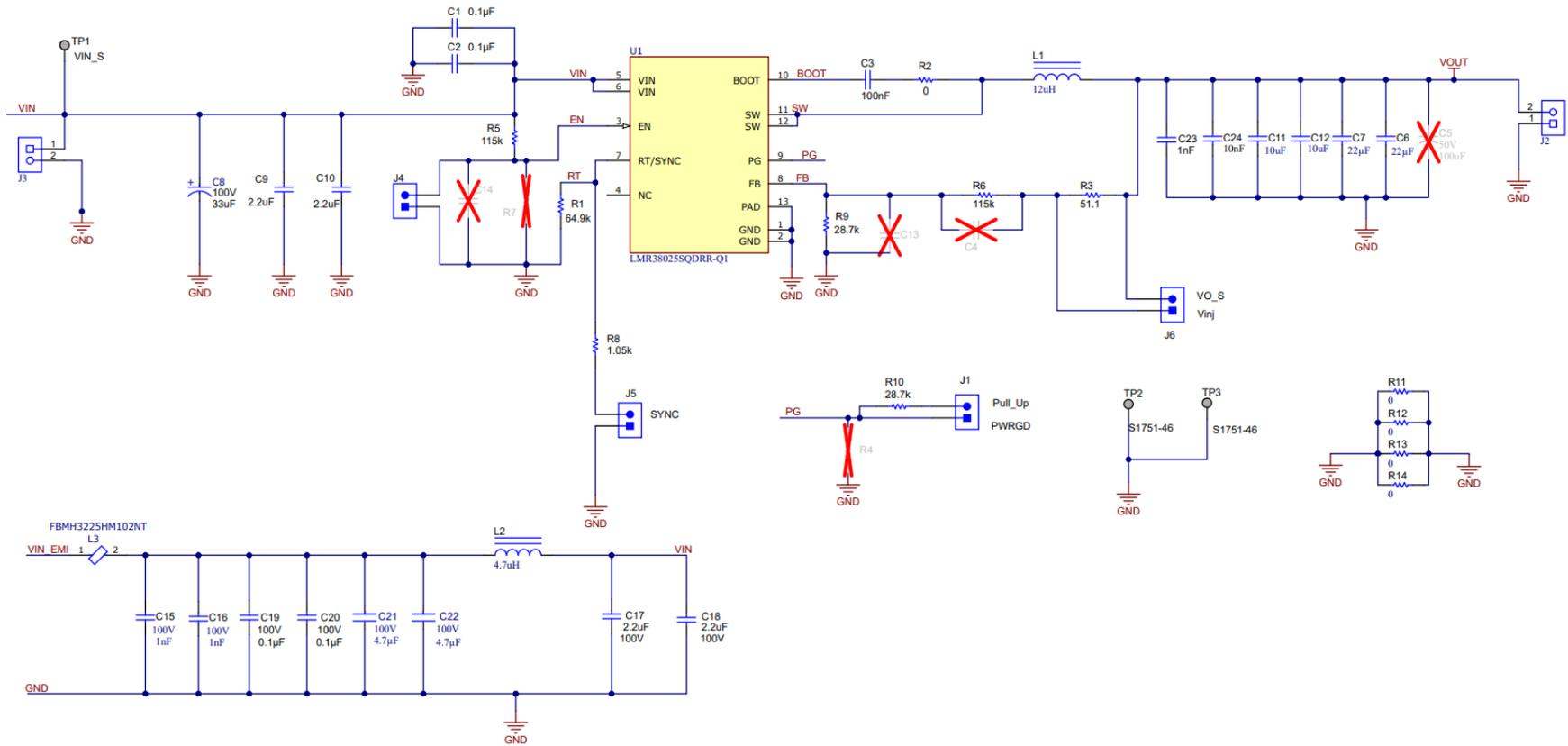
Figure 4-1. LMR38025Q Schematic
