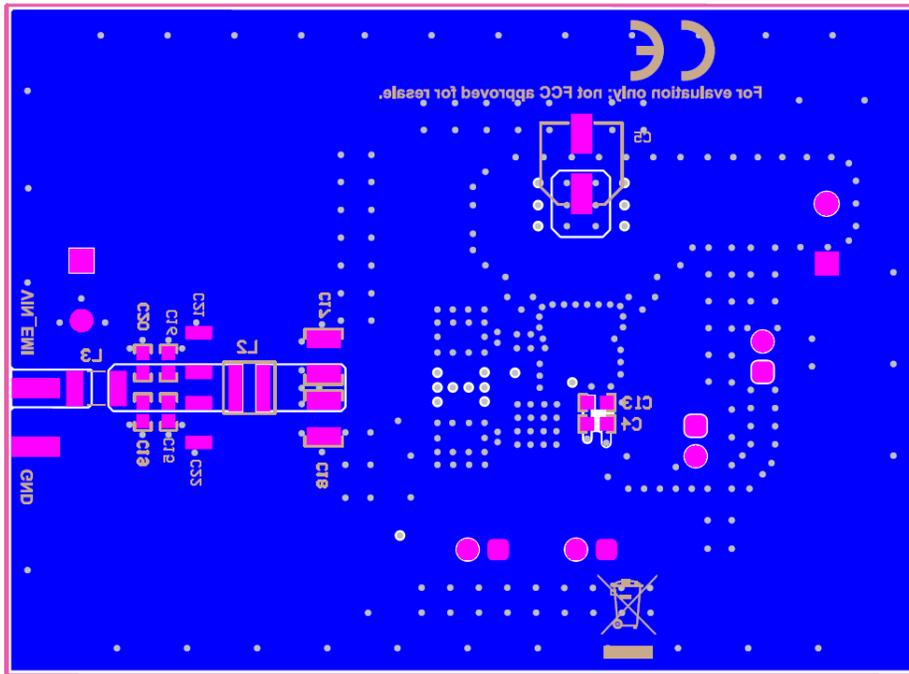
Figure 5-4. Bottom Layer Routing
