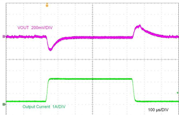
Figure 7-5. Load Transient:  $V_{IN} = 48\text{ V}$ ,  $V_{OUT} = 5\text{ V}$ ,  $I_{OUT} = 250\text{ mA}$  to  $2.25\text{ A}$  at  $200\text{ mA}/\mu\text{s}$
