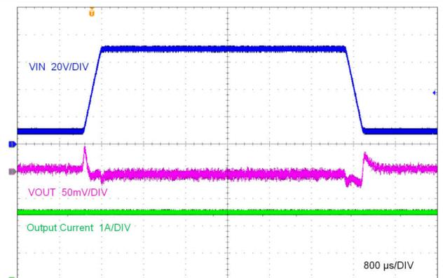
Figure 7-6. Line Transient:  $V_{IN} = 10\text{ V}$  to  $70\text{ V}$  at  $200\text{ V}/\text{ms}$ ,  $V_{OUT} = 5\text{ V}$ ,  $I_{OUT} = 2.5\text{ A}$
