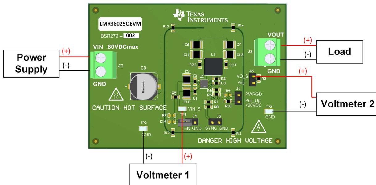
Figure 2-1. LMR38025Q EVM Setup
