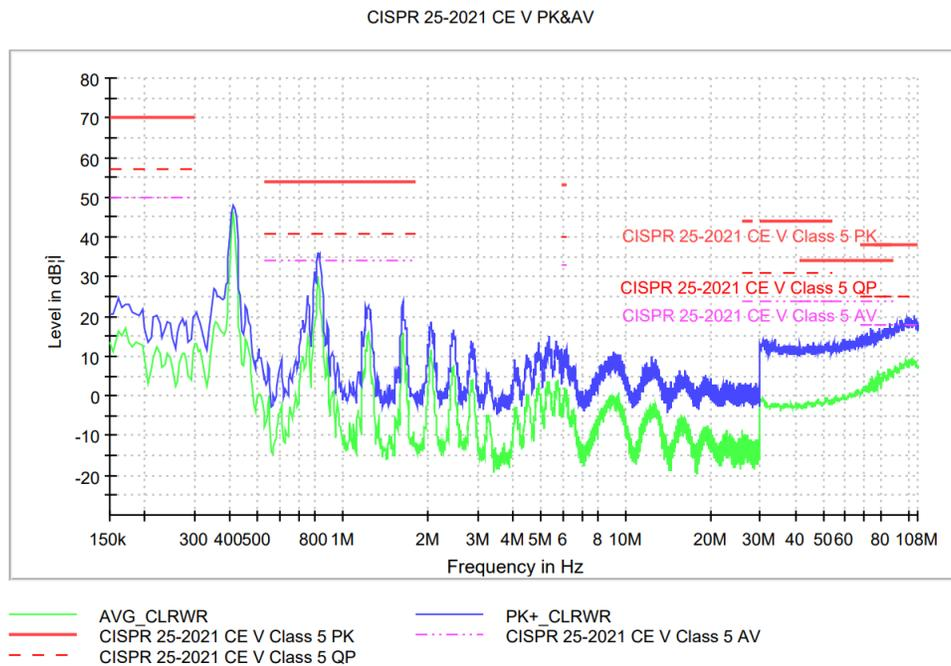
Figure 7-9. CISPR 25 Class 5 Conducted Emissions Plot:  $V_{IN} = 48\text{ V}$ ,  $V_{OUT} = 5\text{ V}$ ,  $I_{OUT} = 2.5\text{ A}$
