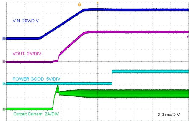
Figure 7-3. Start-Up:  $V_{IN} = 48\text{ V}$ ,  $V_{OUT} = 5\text{ V}$ ,  $I_{OUT} = 2.5\text{ A}$
