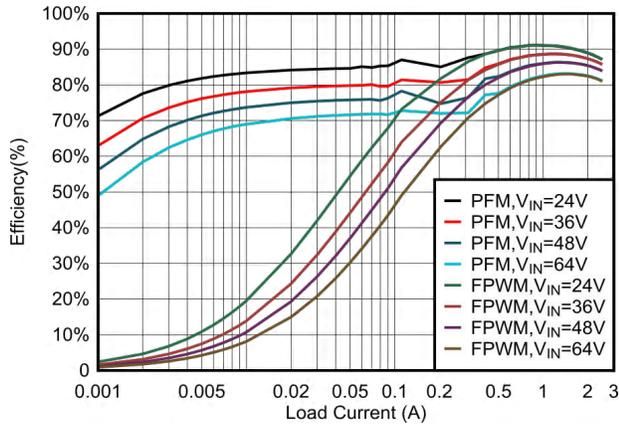
Figure 7-1. Efficiency vs Load Current
