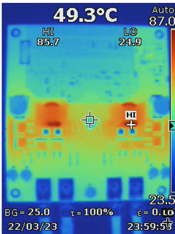
Figure 4-3. Thermal Image: Buck Mode, V_{in}=48V , V_{OUT} = 14.5V , I_{OUT}=60A , Natural Convection
